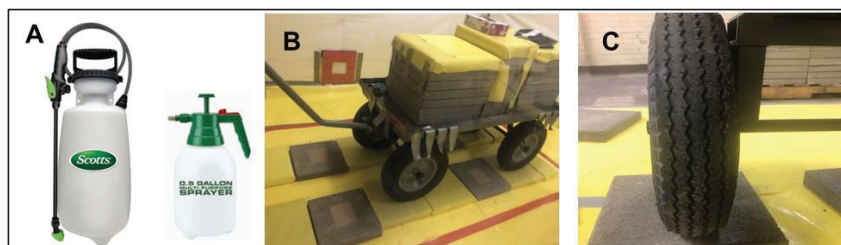
Figure 6. Sprayers Used in Study (A), Wagon Used to Simulate Applicable Vehicle (B), and Simulated Vehicle Tire (C).
