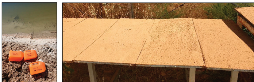
Figure 1. Samples of Dead Sea salt solutions collected in 3 L containers (left side) and trays of Ze'elim soil treated with different brines (surface area of 0.5 \text{ m} \times 1.0 \text{ m} and height of 0.02 \text{ m} ).
