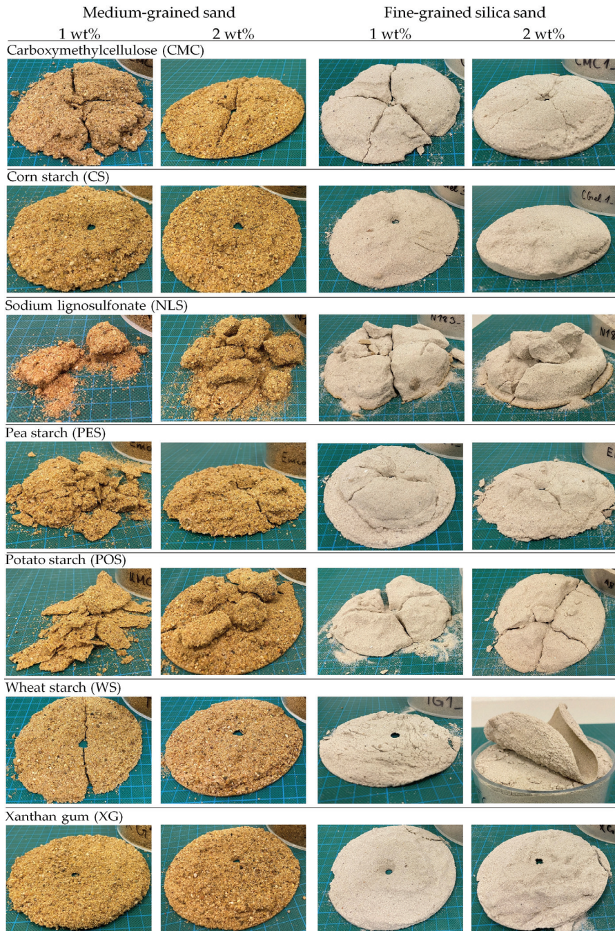
Figure 10. Examples of polysaccharide-induced crusts recovered from the samples (cf. Table A6 for classification).
