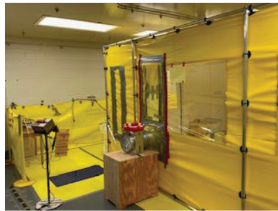
Figure 4. Radiological Containment Tent.
