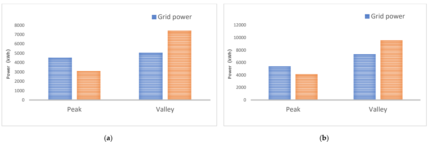
Figure 10. Comparison of the results of peak shaving and valley filling: (a) in summer; (b) in winter.
