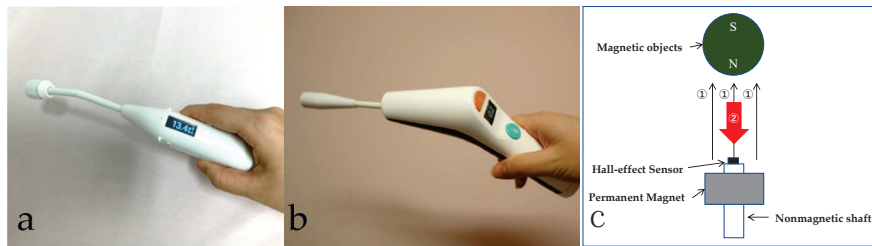
Figure 1. The magnetic probe TAKUMI (Matrix cell Research Institute Inc., Tokyo, Japan): (a) First type: Gen.1; (b) Second type: Gen.2; (c) The detection mechanism of TAKUMI. ① The objects are magnetized by the magnetic fields from the permanent magnet. ② The newly generated magnetic field from the magnetized objects is detected by the Hall effect sensor.
