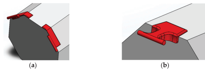
Figure 6. Detail of the clamps: one side of the package is constrained by two clamps (a), and the opposite side is constrained by a single clamp (b).
