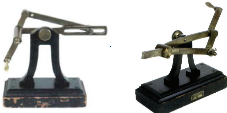
Figure 19. Examples of the iron-made crank-slider mechanism models from the 1930s' within the collection at the Department of Mechanics, Milan.
