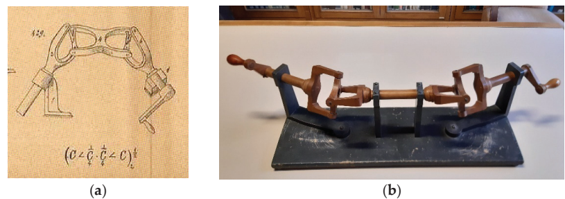
Figure 3. A model of the double Hooke's joint: (a) in the treatise of Masi [34]; (b) the corresponding wooden model at the University of Bologna.
