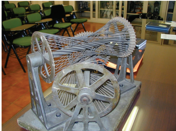
Figure 16. The iron-made model of the hypoid connections representing the screw motion and hypoid gears.
