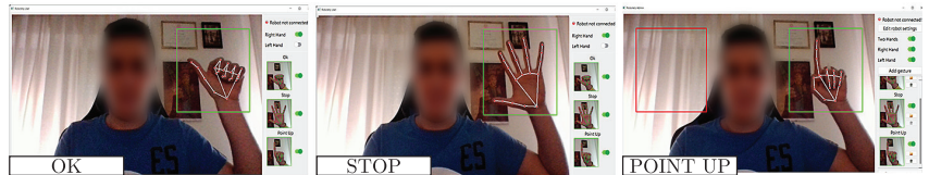
Figure 3. Example of gesture recognition using a standard webcam and Robotely software [32].
