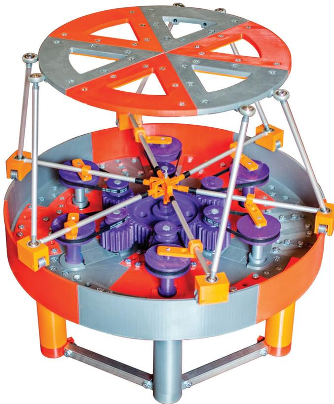
**Figure 6.** The actuated full-scale physical prototype of the proposed hexapod.
