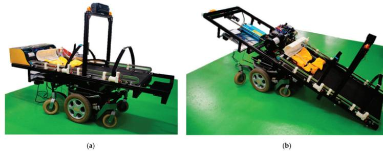
**Figure 10.** The fully assembled ResQbot 2.0. (a) The compact configuration is used for general navigation and casualty transportation. (b) ResQbot 2.0 in the loading configuration, allowing the robot to adjust its configuration to the optimal loading angle to perform the casualty extraction procedure safely.
