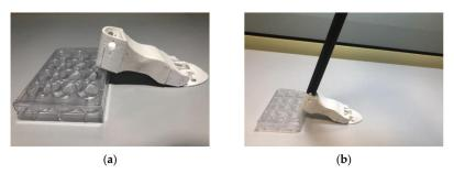
Figure 12. Humanoid foot prototype assembly on a 22 mm step: (a) unloaded test; (b) loaded test.
