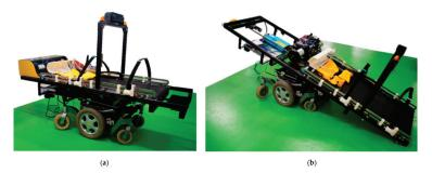
**Figure 10.** The fully assembled ResQbot 2.0. (**a**) The compact configuration is used for general navigation and casualty transportation. (**b**) ResQbot 2.0 in the loading configuration, allowing the robot to adjust its configuration to the optimal loading angle to perform the casualty extraction procedure safely.
