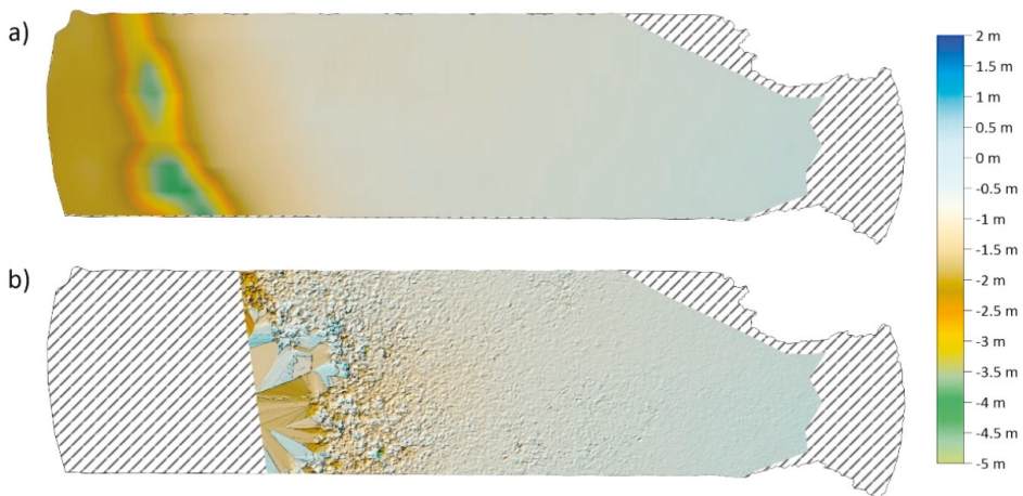
Figure 9. BRS surface developed by the TIN method from USV data in the sounding domain (a) and the corresponding surface developed from UAV data (b). View within the limits of the complete development of the digital bathymetric model.
