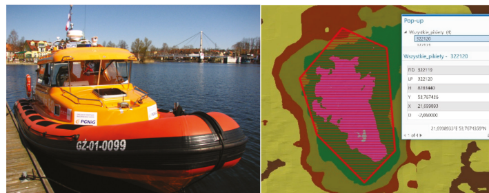
Figure 9. On-site verification of cardinal buoys (measuring platform—Water Rescue Service boat (left), the model with depth readings (right)).
