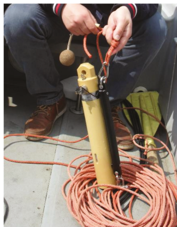
Figure 3. STD/CTD probe model SD204.
