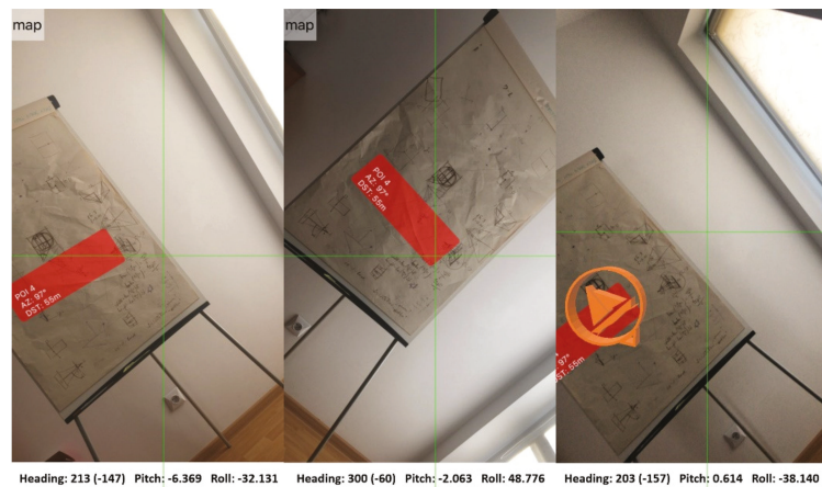
Figure 11. Test application presenting labels and 3D models of spatial objects based on sensor readings.
