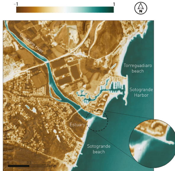
Figure 6. Total climatology (2017–2020) using Sentinel-2 L2A images and NDWI index for the Guadiaro river mouth. Scale 1:15,000.
