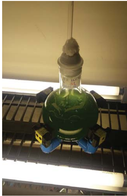
Figure 6. Photograph of the experimental setup for a single flask having the culture inside, surrounded by the permanent magnets, and under illumination.
