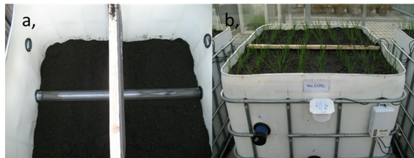
Figure 1. (a) The position of the polycarbonate tubes in the container; (b) The plant stand after the planting.
