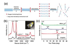
**Figure 3.** (a) Schematic illustration of the intercalation of edge-selective oxidized graphite (EOG); (b) micro-Raman spectra measured at the edge and on the basal plane of EOG; and (c) X-ray diffraction (XRD) of graphite, EOG, graphene oxide (GO) and EOG- $C_{14}$ N<sup>+</sup> intercalated compound. Adapted with permission from [99]. Copyright © 2013 Springer Nature.
