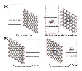
**Figure 4.** (a) The geometric structures of bilayer graphene and CL<sup>+</sup> intercalated bilayer graphene; and (b) the calculated interlayer binding energy of the AB stacking bilayer graphene and CL<sup>+</sup> absorbed bilayer graphene. Adapted with permission from [18]. Copyright © 2017 Elsevier.
