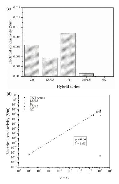
**Figure 6.** Electrical conductivity evolution with filler loading ((**a**) vol % and (**b**) wt %) for CNT series foams and Hybrid series foams; (**c**) comparison of the electrical conductivity of Hybrid series foams; and (**d**) evolution of electrical conductivity with reduced filler loading ( $\phi - \phi_c$ ) assuming a percolative conduction model.
