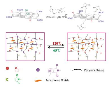
Figure 5. Synthetic routes of nanocomposites. Reproduced with permission from [67]. Copyright (2017) Polymer.
