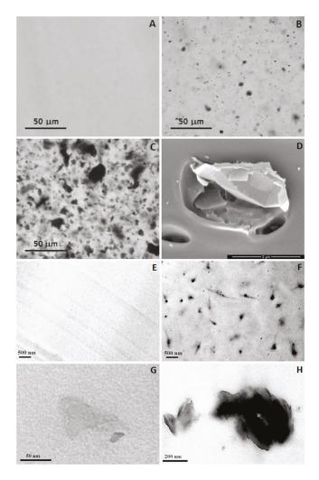
**Figure 3.** Microscopy images of PLA, PLA/GNP and GO 0.4 wt % films produced by solution mixing followed by film casting using doctor blading, displaying good filler dispersion and interaction with polymer matrix. Optical microscopy images of PLA (**A**); PLA/GO (**B**); and PLA/GNP (**C**); Scanning electron microscopy image of PLA/GNP (**D**); Transmission electron microscopy images of PLA (**E**) and PLA/GO (**F–H**) [179].
