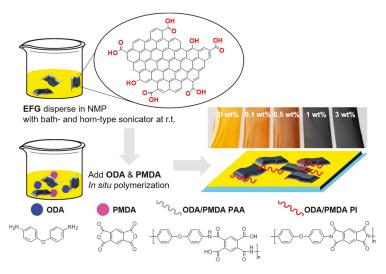
Figure 3. Fabrication process of PI/EFG composites.
