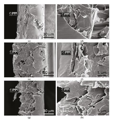
**Figure 3.** SEM images of membranes of: (**a**,**b**) PPO/0.3 wt % of Graphene XT 7; (**c**,**d**) PPO/1 wt % of Graphene XT 6; (**e**,**f**) PPO/5 wt % of Graphene XT 6; and (**g**,**h**) PPO/15 wt % of Graphene XT 6.
