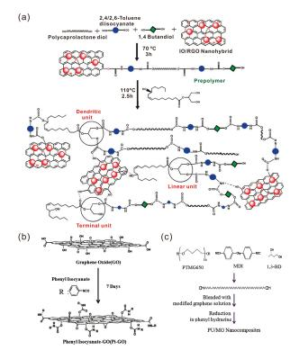
**Figure 4.** (a) Synthesis of a hyperbranched PU/IORGO nanocomposite. Reproduced with permission from [59]. Copyright (2015) New Journal of Chemistry. (b) Modification of graphene oxide (GO) by phenyl isocyanate. (c) Overall reaction scheme to prepare a PU/MG nanocomposite. Reproduced with permission from [62]. Copyright (2013) European Polymer Journal.
