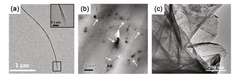
**Figure 13.** TEM images of (a) partially unzipped MWCNTs, inset is the unzipped layer; and (b) graphene nanoribbon (GNR)/epoxy nanocomposites. Adapted with permission from [106]. Copyright © 2016 Elsevier. (c) Polypyrrole (PPy)/GO synthesized by intercalation polymerization. Adapted with permission from [120]. Copyright © 2016 Elsevier.
