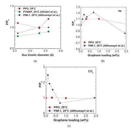
**Figure 10.** (a) Permeability variation induced by graphene addition, as a function of the gas kinetic diameter, in three glassy polymers: PPO (this work), PTMSP [35] and PIM-1 [33]. The weight fraction of graphene added was 1 wt % in the case of PPO and PTMSP; 0.71 wt % in the case of PIM-1. He permeability variation (b); and CO<sub>2</sub> permeability variation (c) after addition of graphene in PPO (this work) and PIM-1 versus graphene loading.
