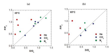
**Figure 8.** Parity plot showing the correlation between the variation of diffusivity induced by addition of graphene and the corresponding variation of permeability at: (a) 35  $^{\circ}$ C; and (b) 65  $^{\circ}$ C.
