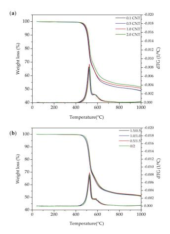
Figure 4. TGA and DTG thermograms of (a) CNT series foams, and (b) Hybrid series foams.
