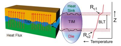
**Figure 7.** Schematic illustrating the action of thermal interface material, which fills the gaps between two contacting surfaces and conducts the heat produced by electronic drives [101]. (Copyright (2012) the American Chemical Society).
