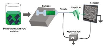
Figure 1. Schematic illustration of the electrospinning setup.
