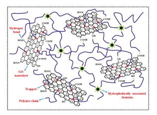
**Figure 3.** A proposed structure illustration of GO/hydrophobically associated polyacrylamide (HAPAM) composite hydrogels. Reproduced with permission from [49]. Copyright (2015) Journal of Materials Chemistry A.
