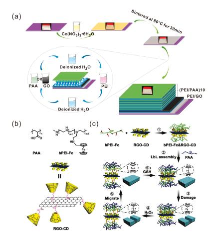
**Figure 6.** (a) Preparation process of the self-healing anticorrosion coating. Reproduced with permission from [75]. Copyright (2015) ACS Applied Materials and Interfaces. (b) The chemical structures of bPEI-Fc, PAA and RGO-CD. (c) Schematic illustration of the fabrication and healing process of the PAA/bPEI-Fc&RGO-CD composite films. Reproduced with permission from [77]. Copyright (2017) ACS Nano.
