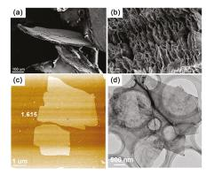
**Figure 11.** SEM images of (**a**) natural graphite and (**b**) expanded graphite; (**c**) atomic force microscope (AFM) image and (**d**) TEM image of PMMA/graphene composites. Adapted with permission from [119]. Copyright © 2017 American Chemical Society.
