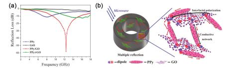
**Figure 16.** (a) The reflection loss (RL) of the samples with a thickness of 2.96 mm; and (b) schematics of electromagnetic waves (EM) loss-enhancement mechanism of PPy/GO. Adapted with permission from [120]. Copyright © 2016 by the Elsevier.
