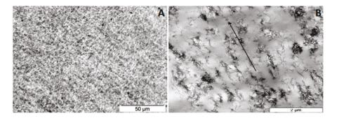
**Figure 4.** Optical microscopy image of a PLA/MWCNT 3 wt % mixture produced by twin-screw extrusion (**A**)—illustrating the high degree of macroscopic filler dispersion. Transmission electron microscopy image of a PLA/MWCNT 3 wt % mixture produced by twin-screw extrusion, followed by piston spinning; (**B**)—arrow indicates that fillers are strongly oriented in fiber direction due to the spinning process [185].
