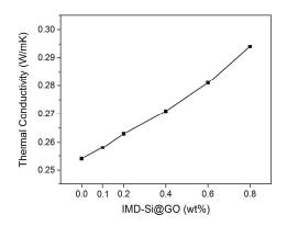
Figure 13. Thermal conductivities of epoxy composites with different contents of IMD-Si@GO fillers.
