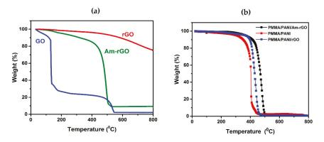
**Figure 8.** TGA curves (**a**) of GO, rGO and Am-rGO; and (**b**) for electrospun PMMA/PANI/Am-rGO, PMMA/PANI/rGO and PMMA/PANI nanofibers.
