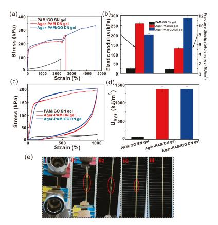
**Figure 11.** (a) Tensile stress–strain curves, and (b) elastic modulus and fracture dissipated energy of a PAM/GO single network (SN) gel, agar-PAM DN gel, and agar-PAM/GO DN gel. (c) Loading–unloading cyclic tensile stress–stain curves at a maximal strain of 1000%, and (d) corresponding dissipated energy of three gels. (e) Photos of the stretching process of agar-PAM/GO DN gel (from i to iii). Reproduced with permission from [48]. Copyright (2016) Advanced Engineering Materials.
