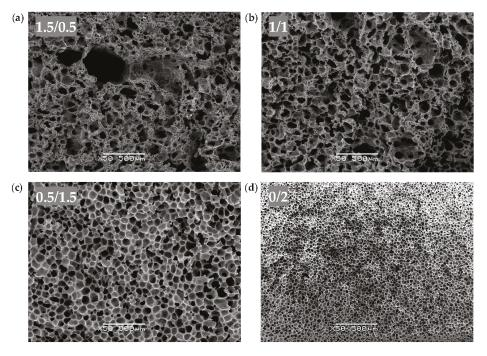
**Figure 2.** Typical SEM images at  $\times$ 50 magnification showing the general cellular structure of the Hybrid series foams: (a) 1.5 wt % CNT and 0.5 wt % GnP, (b) 1.0 wt % CNT and 1.0 wt % GnP, (c) 0.5 wt % CNT and 1.5 wt % GnP, and (d) 0.0 wt % CNT and 2.0 wt % GnP.
