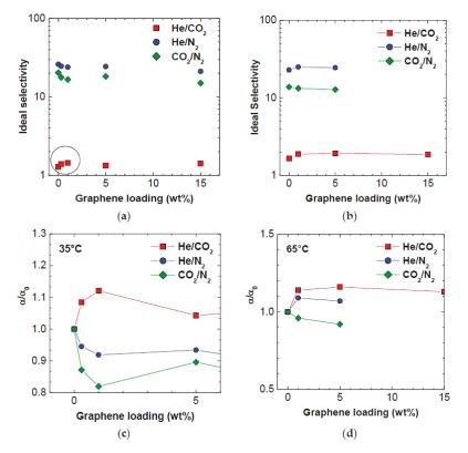
**Figure 6.** Gas ideal selectivity at: (a) 35 °C; and (b) at 65 °C, as a function of graphene loading in PPO. Variation of PPO selectivity after addition of graphene vs. graphene loading at (c) 35 °C and (d) 65 °C.
