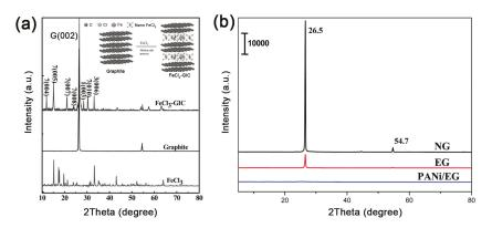
**Figure 10.** (a) XRD patterns of graphite, FeCl<sub>3</sub> and FeCl<sub>3</sub>-GIC; insert is the schematic of graphite and FeCl<sub>3</sub>-GIC. Adapted with permission from [62]. Copyright © 2014 Royal Society of Chemistry. (b) XRD patterns of natural graphite, expanded graphite (EG) and graphene/polyaniline (PANi)/EG hybrids synthesized by intercalation polymerization. Adapted with permission from [53]. Copyright © 2014 Wiley Online Library.
