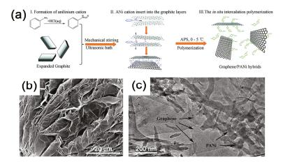
**Figure 8.** (a) Schematic for the in situ intercalation polymerization of ANi<sup>+</sup> into EG to synthesize graphene/polyaniline hybrids; (b) scanning electron microscope (SEM) image of expanded graphite; and (c) transmission electron microscope (TEM) image of graphene/polyaniline hybrids obtained by in situ intercalation polymerization. Adapted with permission from [53]. Copyright © 2014 Royal Society of Chemistry.
