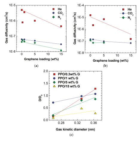
**Figure 7.** Diffusivity of the various gases in the PPO composite membranes at various values of graphene loadings at: (a)  $35 \,^{\circ}$ C; and (b)  $65 \,^{\circ}$ C; (c) Gas-dependent effect of graphene on membrane diffusivity at  $35 \,^{\circ}$ C: the chart shows the relative increase of membrane gas diffusivity after graphene addition versus the size of the gas molecule for various loadings of graphene.
