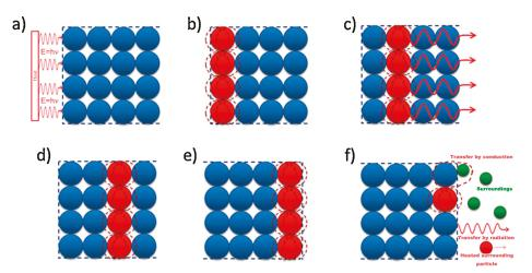
**Figure 1.** The schematic of thermal conductance in a crystalline material [29]. Copyright (2016), with permission from Elsevier.
