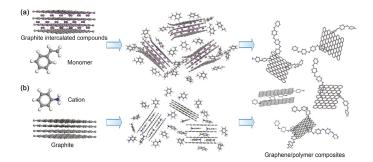
**Figure 5.** Schematic of the two kinds of polymerization in the interlayer of graphite: (**a**) polymerization initiated by pre-intercalated compounds; and (**b**) polymerization initiated after intercalation of monomers (in situ intercalation polymerization).
