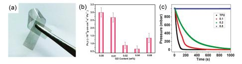
**Figure 19.** (a) Digital image of poly(vinyl alcohol (PVA)/GO composites film synthesized by intercalation polymerization; and (b) its water vapor permeability. Adapted with permission from [107]. Copyright © 2016 Royal Society of Chemistry. (c) Pressure drop curves of thermoplastic polyurethane (TPU)/GNR composites. Adapted with permission from [115]. Copyright © 2013 by the American Chemical Society.
