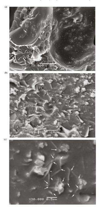
**Figure 8.** (**a**–**c**) Characteristic high magnification SEM images showing nanoparticle dispersion in Hybrid series foams. White arrows in (**c**) show physical contact between nanoparticles.
