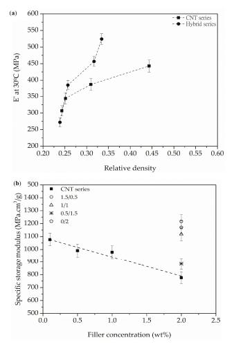
**Figure 5.** (a) Evolution of the storage modulus (*E'*) measured at 30 °C with increasing relative density and (b) evolution of the specific storage modulus at 30 °C with increasing filler concentration for CNT series foams and Hybrid series foams.
