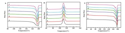
**Figure 7.** Differential scanning calorimetry (DSC) curves of the first heating process (**A**), cooling process (**B**), and the second heating process (**C**) for different samples. PLLA (a), GO-g-PLLA0.3/PLLA (b), GO-g-PLLA0.7/PLLA (c), GO-g-PLLA1/PLLA (d), GO-g-PLLA3/PLLA (e), and GO-g-PLLA5/PLLA (f).
