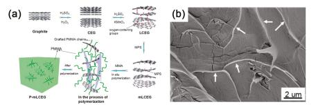
**Figure 9.** (a) Schematic of the preparation of polymethyl methacrylate (PMMA)/graphene composites by interlayer polymerization; and (b) SEM image of freeze-fractured cross sections of composites. Adapted with permission from [119]. Copyright © 2017 American Chemical Society.
