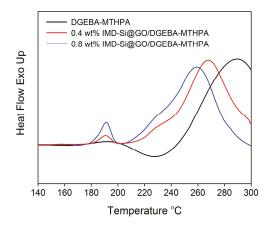
Figure 12. DSC curing curves of epoxy resin-anhydride with different contents of IMD-Si@GO with a heating rate of 10 °C/min.
