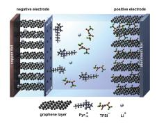
**Figure 2.** Schematic illustration of a dual-graphite cell with no effective solid electrolyte interphase layer at the graphite anode during the charge process. The negative graphite electrode suffers from exfoliation reactions caused by co-intercalation of the relatively large  $Pyr_{14}^+$  cations [82]. Published by The Royal Society of Chemistry.
