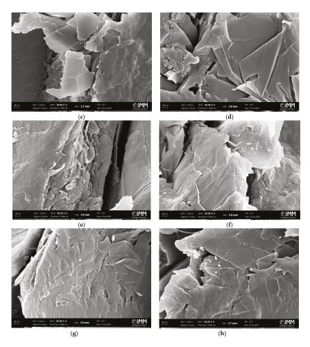
**Figure 4.** SEM images of membranes of: (**a**,**b**) PPO/0.3 wt % of Graphene XT 7; (**c**,**d**) PPO/1 wt % of Graphene XT 6; (**e**,**f**) PPO/5 wt % of Graphene XT 6; and (**g**,**h**) PPO/15 wt % of Graphene XT 6.
