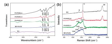
**Figure 12.** (a) Fourier-transform–infrared (FT–IR) and (b) Raman spectra of expanded graphite (EG), PANi and PANi/EG composites. (PANi/EG grinding mixture was denoted as PANi/EG-0, the intercalation polymerization and in situ polymerization of ANi<sup>+</sup> into 1 wt % EG was denoted as PANi/EG-1 and PANi/EG-2, respectively.) Adapted with permission from [53].Copyright © 2014 Royal Society of Chemistry.
