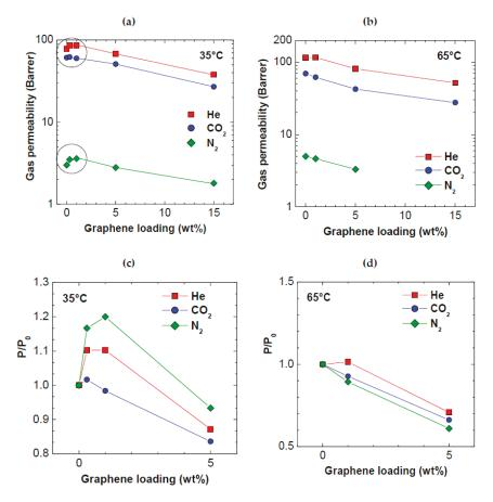
**Figure 5.** Gas permeability at: (a) 35 °C; and (b) at 65 °C, as a function of graphene loading in PPO. Variation of PPO permeability after addition of graphene vs. graphene loading at: (c) 35 °C; and (d) 65 °C.
