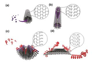
**Figure 6.** Reaction scheme of multiwalled carbon nanotubes (MWCNTs) unzipping and edge-selective in situ polymerization of vinyl monomers. (**a**) Intercalation of MWCNTs by potassium naphthalenide; (**b**) formation of longitudinal fissure in the walls; (**c**) polymerization of styrene assists in exfoliation of MWCNTs; (**d**) polymer functionalized GNRs. Adapted with permission from [110]. Copyright © 2013 American Chemical Society.
