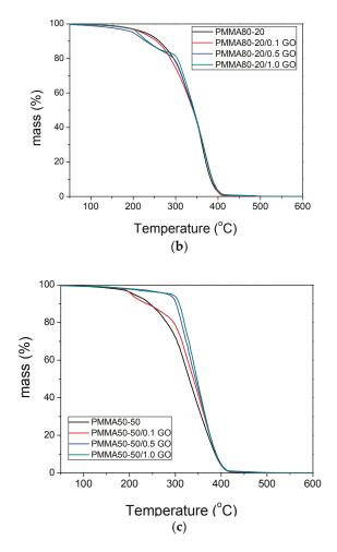
**Figure 9.** Mass loss of neat PMMA and PMMA/GO nanocomposites with various amounts of added GO obtained in bulk (**a**); solution with 80–20 (**b**); 50–50 (**c**) ratio of monomer to solvent.
