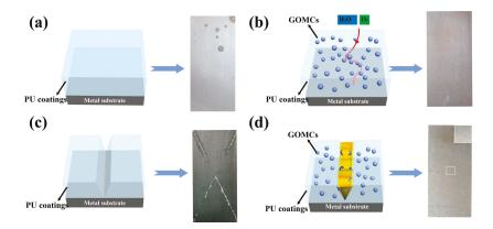
**Figure 14.** Schematic and images of (**a**) neat PU coating and (**b**) GOMCs/PU coatings subjected to the salt spray test for 116 h. Schematic and images of (**c**) neat PU coating and (**d**) GOMCs/PU coatings after scratching and 15 days of healing, subjected to the salt spray test for 43 h. Inset: the enlarged view of the white block. Reproduced with permission from [36]. Copyright (2016) Composites Science and Technology.
