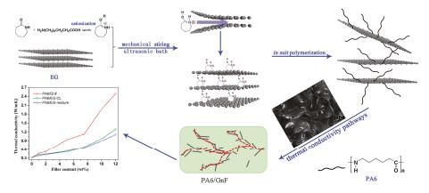
**Figure 18.** Schematic for the in situ intercalation polymerization of CL<sup>+</sup> into EG to synthesize polyamide-6/graphite nanoflakes composites. Adapted with permission from [18]. Copyright © 2017 Elsevier.
