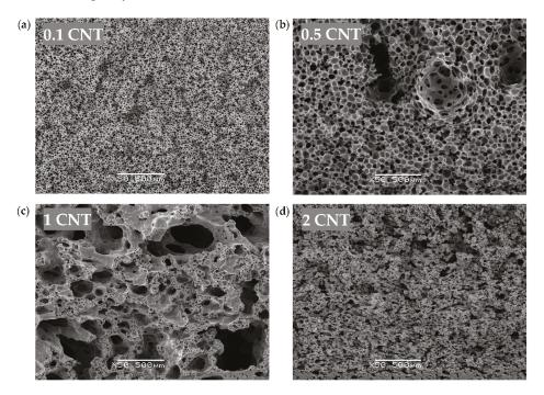
**Figure 1.** Typical SEM images at  $\times$ 50 magnification showing the general cellular structure of the CNT series foams: (a) 0.1 wt %, (b) 0.5 wt %, (c) 1.0 wt %, and (d) 2.0 wt % of CNT.
