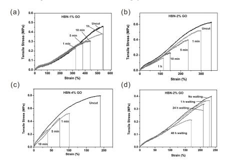
**Figure 9.** Strain-stress curves of the self-healing composites with GO at (**a**) 1 wt %, (**b**) 2 wt % and (**c**) 4 wt % (termed HBN-1% GO, HBN-2% GO, HBN-4% GO, respectively) upon different healing time at room temperature; (**d**) Strain-stress curves of the HBN-2% GO samples of 10 min healing at different waiting time. The waiting was performed at approx. 0% relative humidity from [99]. Copyright (2013) Advanced Materials.
