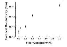
Figure 8. Electrical conductivity of neat PI and PI/EFG composites.
