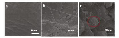
**Figure 6.** Scanning electron microscopy (SEM) images of the tensile failure section for PLLA (**a**), GO-g-PLLA3/PLLA (**b**) and GO-g-PLLA5/PLLA (**c**). Images in the red circle demonstrates the aggregation of nanofiller.
