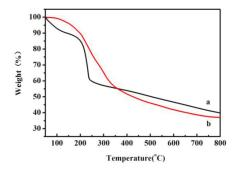
Figure 3. Thermal degradation curves of GO (a) and GO-g-PLLA (b).
