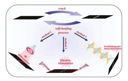
**Figure 10.** The graphene-thermoplastic PU composites were healed by IR light, electricity and electromagnetic waves with high healing efficiencies. Reproduced with permission from [91]. Copyright (2013) Advanced Materials.
