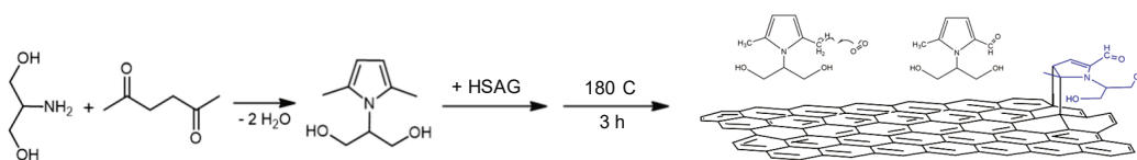
Figure 3. Scheme of the domino reaction for the functionalization of HSAG with serinol pyrrole.
