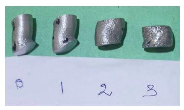
Figure 17. Distorted compression test specimens.
