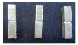
Figure 4. Impact test specimen.
