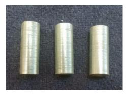
Figure 3. Compressive test specimens.
