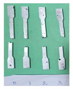
Figure 13. Fractured tensile test specimens.
