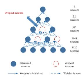
Figure 7. The structure of the adopted DNN with LCTD features and the dropout technique.
