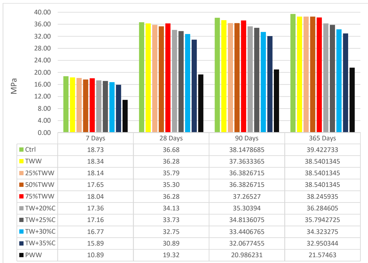
Figure 4. Compressive strength cured by treated wastewater.
