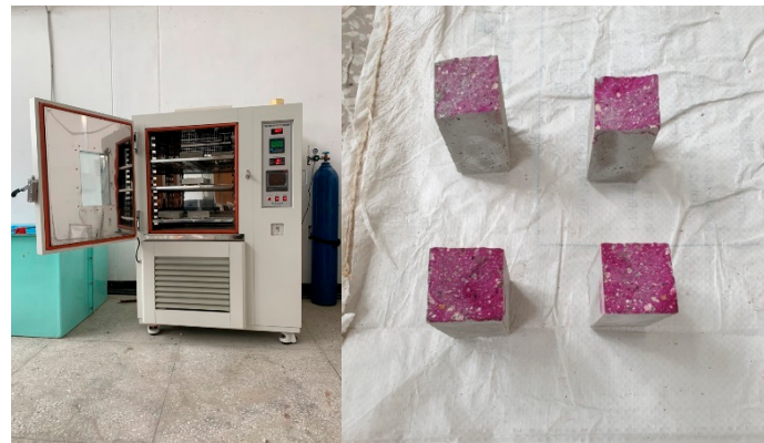
Figure 3. Accelerated-carbonation chamber and samples.
