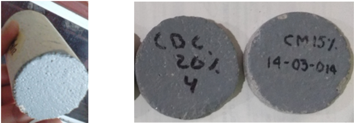
Figure 2. Vinyl paint applied in cross sections of cylinders.
