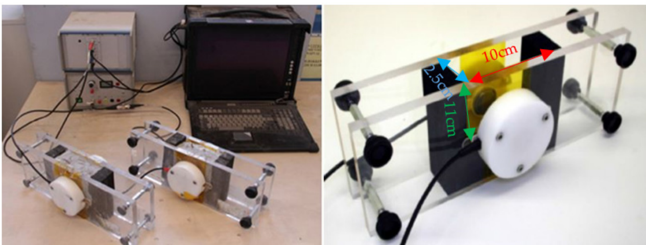
Figure 1. FreshCON system [63] for measuring the ultrasonic pulse velocity.
