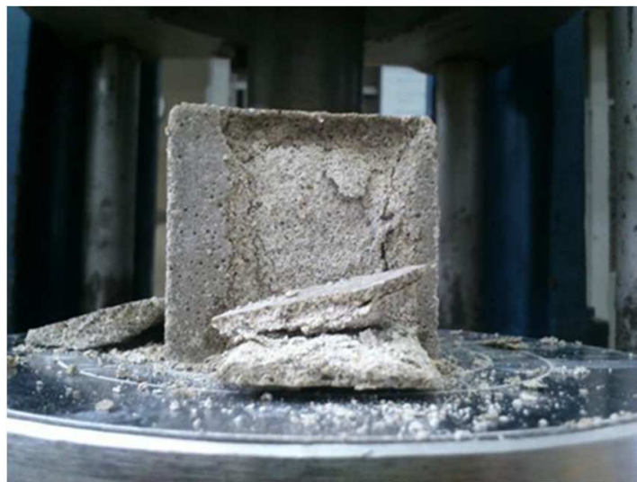
Figure 4. Illustration of the compressive strength test.
