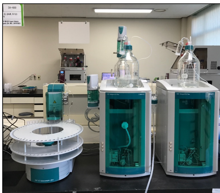
Figure 6. 930 Compact IC Flex ion chromatography (940 Compact IC Flex, Metrohm, FL, USA).
