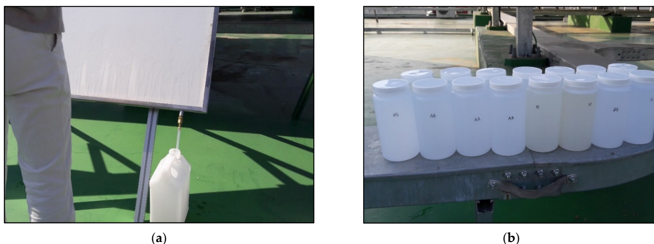
Figure 12. Collecting process and storage procedure of washing water. (a) collecting process of washing water; (b) collected washing water in separate bottles.
