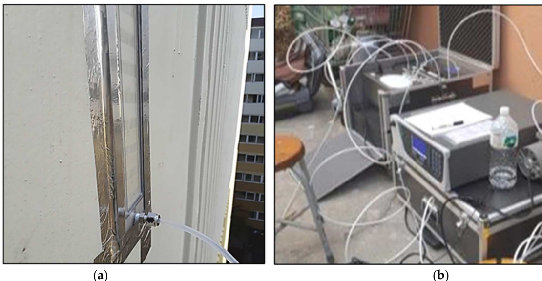
Figure 3. The experimental setup of photoreactor experiment on the wall. (a) Photoreactor with NO gas injection hoses on the eastern wall; (b) portable analysis device for NOx removal.
