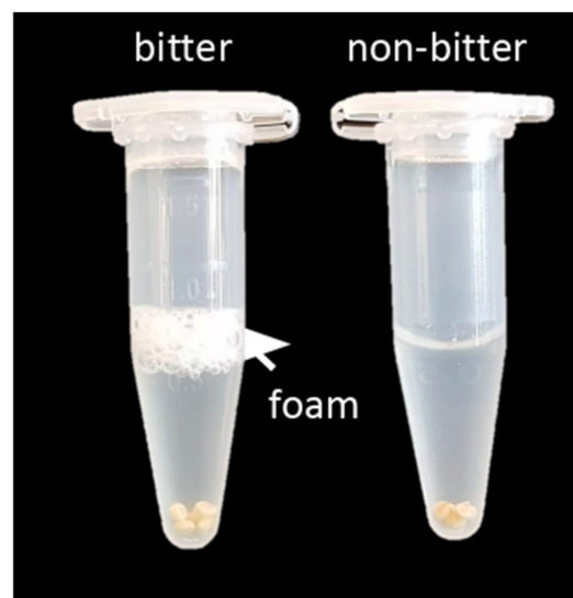
Figure 10. Foaming test (afrosimetric method) for presence or absence of saponins on quinoa seeds.
