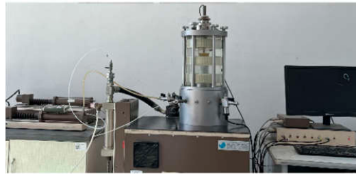
Figure 3. Dynamic triaxial test loading system.
