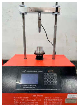
Figure 2. UCS test system.
