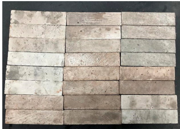
Figure 5. Specimens of fiber-reinforced recycled-brick-powder cementitious composite.
