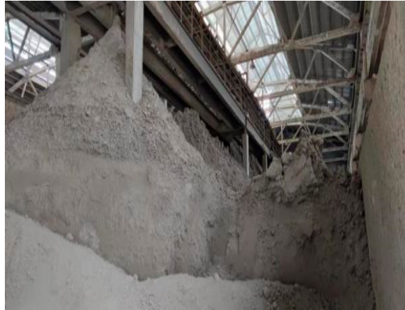
Figure 1. Iron-ore tailings for test.
