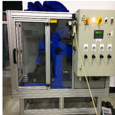
Figure 4. Vibratory roller compacting machine.
