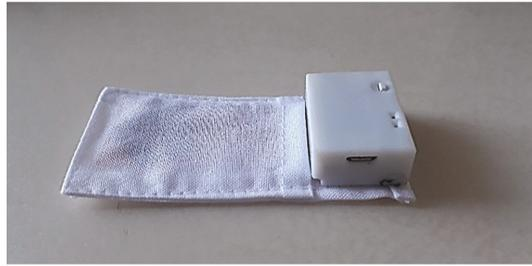
Figure A2. The pulse radar sensor.
