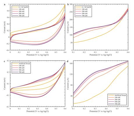
Figure 6. Electrochemical analysis of fully printed Cu<sub>2</sub>O-based glucose sensors over a glucose concentration range of 100–700  $\mu$ M. (a) CV and (b) DPV in 0.1 M NaOH. (c) CV and (d) DPV artificial sweat in 0.1 M NaOH.
