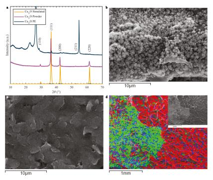
**Figure 2.** (a) XRD spectrum of simulated  $Cu_2O$ , synthesized powder  $Cu_2O$ , and WE drop casted with  $Cu_2O$  nanoclusters ( $Cu_2O$  PE). (b) SEM images of the  $Cu_2O$  drop casted on the PEs: (b)  $Cu_2O$  nanoclusters, (c) graphene paste and (d) EDS mapping of the interface between  $Cu_2O$  and the graphene paste with an inset of the SEM image. Green corresponds to Cu, blue to O, and red to C.
