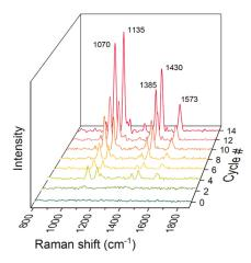
Figure 6. SERS spectra showing an increment in each peak of 4-ATP (12.5 ppm) with increasing number of LbL cycles.
