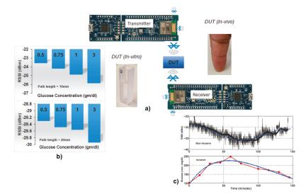
Figure 5. (a) Experimental set-up for both the *in-vitro* and *in-vivo* measurements with a bluetooth enabled MCU (Antenna as Sensors) (b) The RSSI power level dependence on glucose concentration with *in-vitro* experiment (c) Comparison with *in-vivo* experimental results of the noninvasive device with the blood-pricking invasive technique following OGTT protocol on a human subject. Reproduced with permission [107]. Copyright 2019 IEEE.
