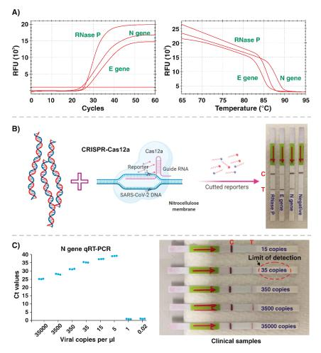
**Figure 1.** (**A**) RT-LAMP reaction performed in an RT-qPCR machine using N, E, and RNase P primers at an optimal temperature and time. (**B**) Schematic illustration of CRISPR-Cas12a reaction on pre-amplified SARS-CoV-2 target genes, followed by visualization with lateral flow strips. (**C**) The detection limit of the RT-qPCR assay (left) using PCR machine and RT-LAMP/Cas12a assay (right) using clinical samples.
