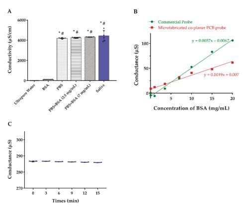
**Figure 4.** (**A**) Conductivity of the solution with different components. (**B**) Detection of the conductance of ultrapure water spiked in with BSA comparing our co-planar microelectrode and the commercial electrode. (**C**) Serial conductance measurements of the 6 individuals' saliva at different time points. Abbreviations: BSA, bovine serum albumin; PBS, phosphate-buffered saline. \* indicates p < 0.05 compared to ultrapure water; # indicates p < 0.05 compared to the BSA.
