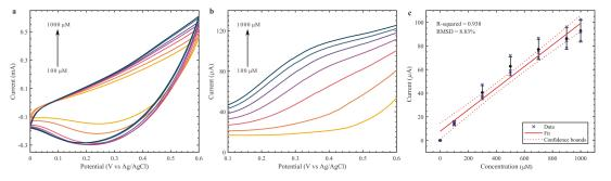
**Figure 4.** CV (a) and DPV (b) of Cu<sub>2</sub>O nanoclusters on printed WE with varying glucose concentrations (100–1000  $\mu$ M) in 0.1 M NaOH. (c) Calibration curve at 0.35 V from DPV analysis.
