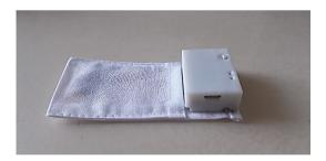
Figure A2. The pulse radar sensor.
