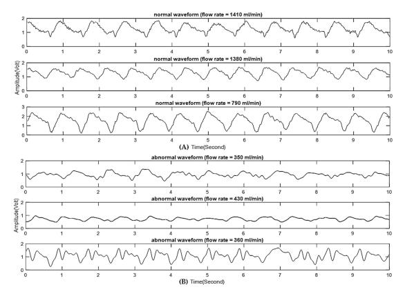
Figure 2. (A) Baseband signals of normal AVF with stable and consistent VWM waveforms. (B) Baseband signals of abnormal AVF with unstable and superimposed oscillations on VWM waveforms.
