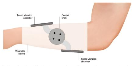
purely mechanical, eliminating the need of a power source. Preliminary results showed an 85% tremor suppression in a patient with PD tremors [115]. Recruitment for a pilot clinical study is ongoing, which should provide further data.
