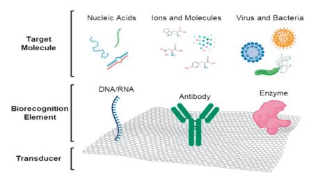
**Figure 2.** A typical saliva-based biosensor. Briefly, it consists principally of three components, a surface (carbon-based or metal) to accommodate the biorecognition element (probes, antibodies, or enzymes), which captures the target (genomic material, antibodies, proteins, etc.). The molecular interactions induce colorimetric or spectrometric changes, which can be observed with their corresponding detection technologies. Image used with permission from Goldoni et al., 2021 [63].
