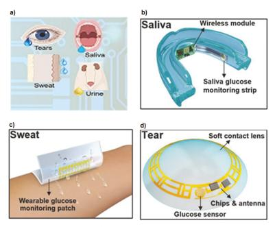
Figure 6. (a)The important bio-fluids like tears, saliva, sweat, and urine used to build non-invasive glucose monitoring devices. Typical biosensors based on (b) saliva, (c) sweat and (d) tear. Reproduced with permission [108] Copyright 2022, Ivyspring International Publisher under CC BY. Reproduced with permission [109] Copyright 2018, John Wiley & Sons.
