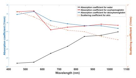
**Figure 2.** Other optical properties values in the utilized in MCS model: scattering coefficients  $\mu_s$  and absorption coefficients for water ( $\mu_a^{H_0O}$ ), deoxyhemoglobin ( $\mu_a^{Hb}$ ), and oxyhemoglobin ( $\mu_a^{HbO_2}$ ) [27,31,38].
