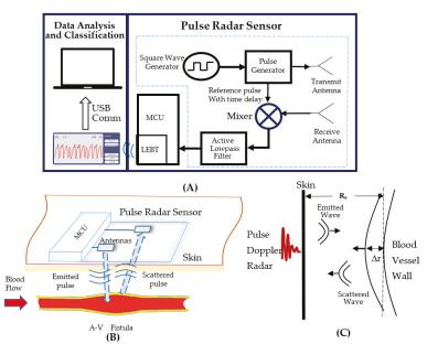
**Figure 1.** The system diagram of the VWM monitor and the principle of measuring the AVF vessel wall movement (**A**). The diagram of pulse radar sensor detect blood flow (**B**). The diagram of pulse Doppler radar emit and receive the signals of wave (**C**).
