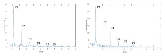
Figure 4. FFT spectrum of normal AVF wall motion signal (left), FFT spectrum of abnormal AVF wall motion signal (right).
