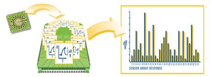
**Figure 1.** Working principle of Cyranose 320: it is based on a nano-composite array of 32 organic polymer sensors. If exposed to VOC combinations, the polymers swell, thereby modifying their electrical resistance. Raw data are registered as the increase in resistance of any single sensors and the combination of all signals results in a "breathprint".
