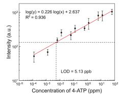
**Figure 7.** SERS intensity at  $1070 \text{ cm}^{-1}$  obtained from a series of different concentrations of 4-ATP dropped onto prepared SERS substrates (analyte concentration ranging from 0.00125 ppm to 12.5 ppm).
