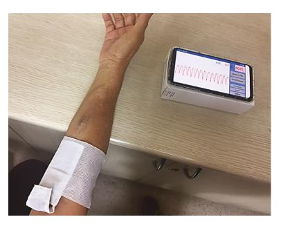
**Figure 3.** The hemodialysis patient during testing using a pulse radar sensor. Note that the App displays the signal waveform on a mobile phone. The detailed strategy of immobilizing as developed by the VWM monitoring system on patients, shown in Appendix A.
