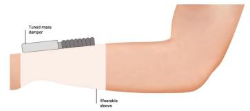
**Figure 4.** Steadi-One passive orthosis. The non-Newtonian fluid within the tuned mass damper of Steadi-One (Steadiwear, Toronto, ON, Canada) becomes viscous when the vibration energy of tremor is transferred to a mass-spring-damper system, acting as a dissipating element that reduces the amplitude of motions.
