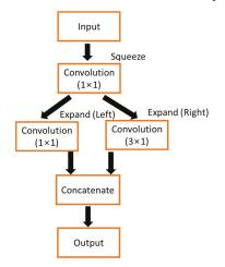
Figure 2. Structure of the proposed fire module of Squeeze U-net.
