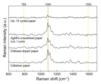
**Figure 5.** Raman spectra obtained from original cellulose, chitosan-doped, LbL 1-cycle, and LbL 14-cycle substrates, where the yellow bands represent the chemical motifs of the following: glycosidic ring stretching, 1090 cm<sup>-1</sup>; amine group in chitosan, 1593 cm<sup>-1</sup>; and silver, 789 cm<sup>-1</sup>.
