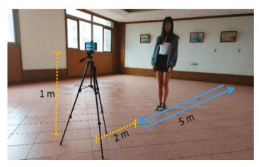
**Figure 2.** Experimental setup (the cell phone was placed 1 m above the floor and 2 m from the participant).
