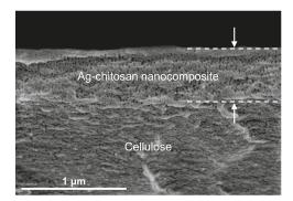
Figure 4. Cross-sectional view of Ag-chitosan nanocomposite on the cellulose substrate (thickness of Ag-chitosan nanocomposite, approx. 575 nm; diameter of nanopores, up to 30 nm).
