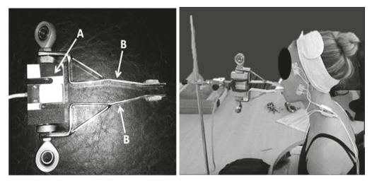
Figure 1. The adapted load cell. (A) laboratory-grade load cell; (B) adapted arms.
