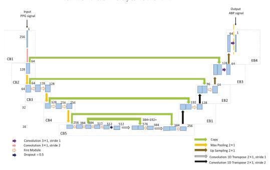
Figure 3. The proposed architecture of one-dimensional (1D) Squeeze U-net DL model.
