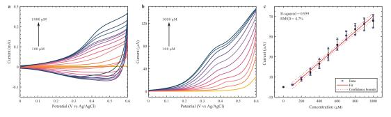
Figure 3. CV (a) and DPV (b) of Cu<sub>2</sub>O nanoclusters on GCE with varying glucose concentrations (100–1000  $\mu$ M) in 0.1 M NaOH. (c) Calibration curve at 0.35 V from DPV analysis.
