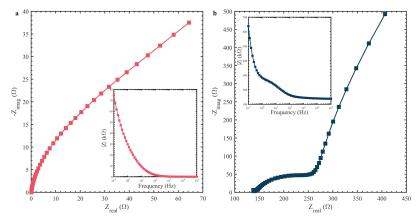
Figure 5. Nyquist plot of 0.1 M NaOH with 100  $\mu$ M glucose solution of (a) Cu<sub>2</sub>O coated GCE with magnitude of impedance inset and (b) Cu<sub>2</sub>O coated on PE with magnitude of impedance inset.
