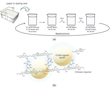
**Figure 1.** (a) Schematic illustration of the layer-by-layer process used to coat cellulose paper with silver/chitosan nanocomposite, where the paper substrate was submerged in each reagent solution, stepwise; (b) Configured silver/chitosan nanocomposite by coordinate bonds between citrate-capped silver nanoparticles and self-assembled chitosan.
