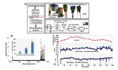
Figure 2. (a) Experimental set up of NIR spectroscopy with LED (b) *In-vitro* NIR spectra of glucose in water solution. Light absorption is proportional to glucose concentration (Inset). (c) *In-vivo* results from experiments on a human subject. Comparison of the transmittance and diffused reflectance techniques with the blood-pricking invasive technique following OGTT protocol. Reproduced with permission from [49]. Copyright 2018, IEEE.
