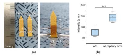
**Figure 8.** (a) Photograph of LbL paper substrate cut into an arrow shape with a lateral transportation and detection zone where the sample liquid moves and is vaporized, consequently focusing analyte molecules on the tip; (b) Signal enhancement by simply cutting the LbL paper substrate (black dot, mean; black solid line in box, median; box height, sample variability from 25% to 75%; error bar, standard deviation; \*\*\* p < 0.001).
