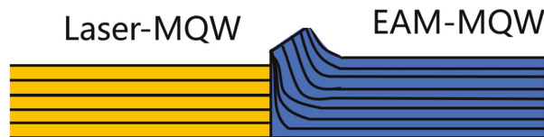
Figure 19. Schematic of the EAM and laser MQWs achieved using the butt-joint technique.
