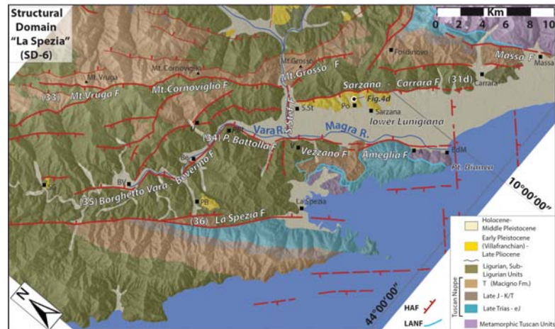
Figure 10. Main fault systems and geology in the structural domain SD6 (La Spezia–lower Lunigiana). The map is derived from [58,107] and our work. Fault identification numbers are as reported in Table S1. HAF: steep normal faults; LANF: low-angle detachment faults; A: Ameglia; BdM: Bocca di Magra; Be: Beverino; BV: Borghetto Vara; PB: Pian di Barca; PBT: Piano Battolla; Po: Ponzano Magra; SG: Sesta Godano; S.St: Santo Stefano Magra; U: Usurana; V: Vezzano.
