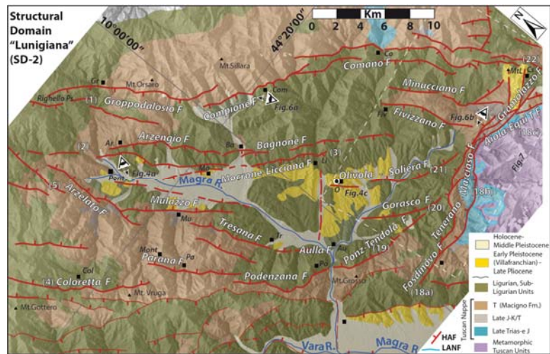
Figure 3. Main fault systems and geology in structural domain SD2 (Lunigiana). The map is derived from [57–60] and our work. Fault identification numbers are as reported in Table S1. HAF: steep normal faults (thicker lines for those described); LANF: low-angle detachment faults; Ar: Arzenio; Au: Aulla; Ba: Bagnone; Co: Comano; Col: Coloretta; Com: Compione; Cs: Castagnola; Fiv: Fivizzano; Gr: Gropodalosio; Li: Licciana; Mont: Montereggi; MtL: Mt. Lupacino; O: Olivola; Pa: Parana; Po: Podenzana; Pont: Pontremoli.
