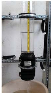
Figure 2. The apparatus and arrangement for testing the hydraulic conductivity of pervious concrete sample.
