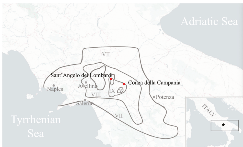
Figure 1. Isoseismal lines of the 1980 earthquake and localization of the two studied towns (modified after Postpischl et al. [13]).
