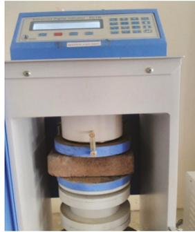
Figure 4. Compressive strength testing of samples.
