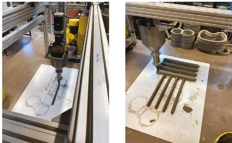
**Figure 1.** Test specimen printing process.
