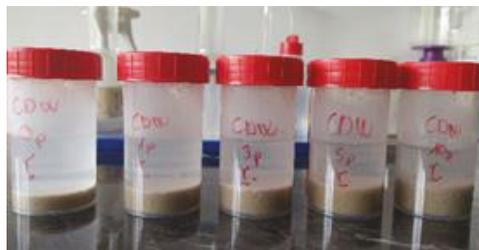
**Figure 2.** CDW samples after the lime sorption test (from left to right: 0 min, 1 min, 3 min, 5 min and 10 min).
