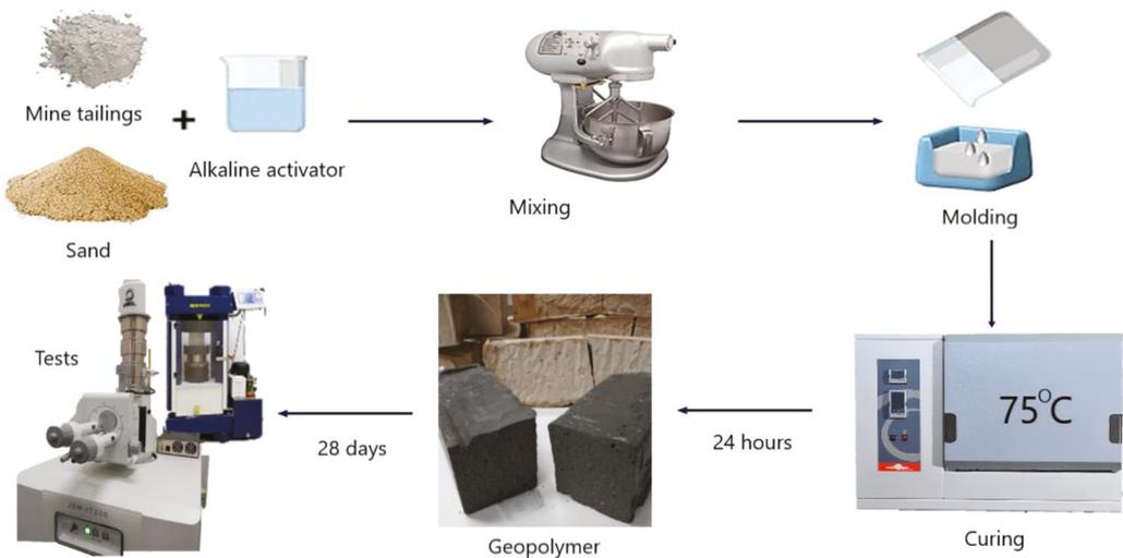
**Figure 1.** Scheme for sample preparation.
