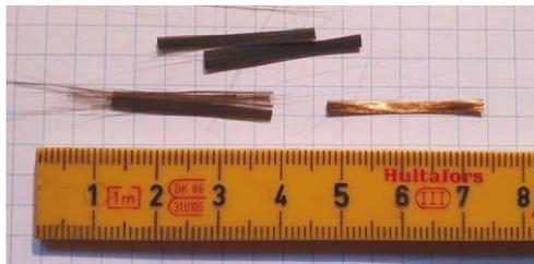
Figure 2. The Basaltex fibers.
