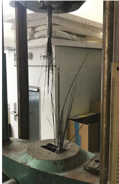
**Figure 4.** Specimen after failure in tension.
