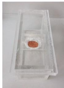
**Figure 4.** One of the model plexiglass boxes for experiments with calcium diffusion.
