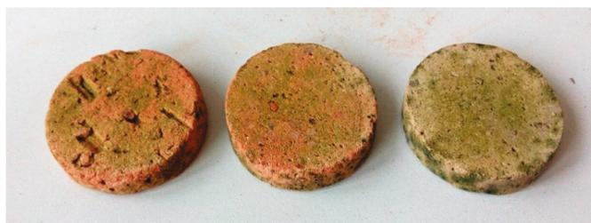
**Figure 7.** Samples of the Holešov-Žopy bricks covered by a biofilm layer of 0–1 cm, 1–2 cm and 2–3 cm (from left to right).
