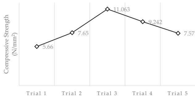
Figure 5. Compressive strength results for brick samples.
