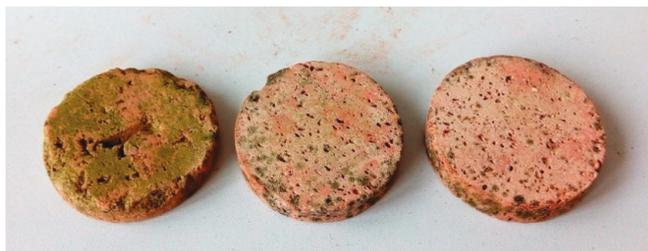
**Figure 5.** Samples of the Vysoké Mýto bricks covered by a biofilm layer of 0–1 cm, 1–2 cm and 2–3 cm (from left to right).
