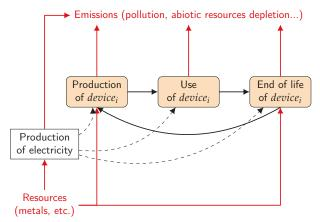
(b) Life cycle phases of each *device*<sub>i</sub> used by the service
