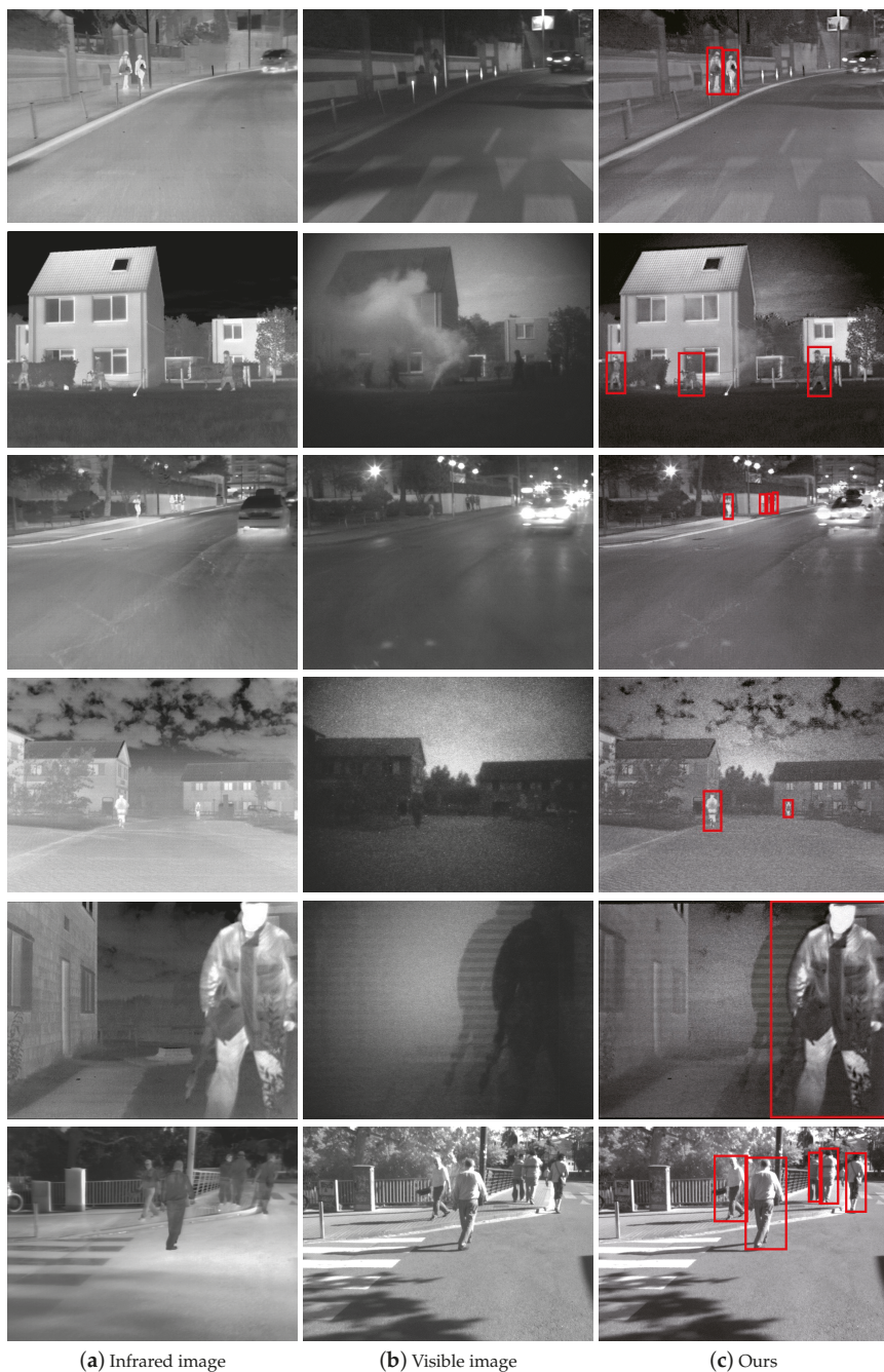
Figure 12. (a–c) Some detection results from our detection network. In order to better display the results, the detection results are shown on the fused images. The images in the first three rows have very low contrast; the objects in the fourth row are relatively small; the object in the fifth row is relatively large; and the images in the last row are in the daytime.
