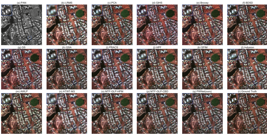
Figure 6. Visual comparison of the CS-based and MRA-based methods and the proposed PWNNet method on the GeoEye-1 images, (a) PAN; (b) LRMS; (c) PCA; (d) GIHS; (e) Brovey; (f) BDSD; (g) GS; (h) GSA; (i) PRACS; (j) HPF; (k) SFIM; (l) Indusion; (m) AWLP; (n) ATWT-M3; (o) MTF-GLP-HPM; (p) MTF-GLP-CBD; (q) PWNNet (ours); (r) Ground Truth.
