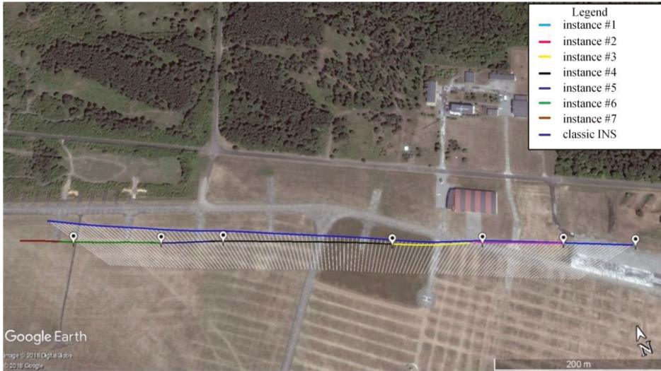
Figure 20. MINS trajectories for flight no 2 (multicolor r line) and INS trajectory (blue line).
