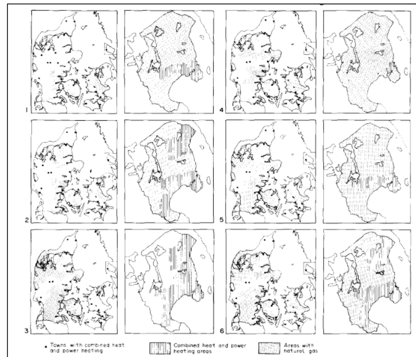
Figure 7. Proposals for regionalization/zoning of heat supply by type of heat supply system. Source: [25]. Notes: The process of zoning comprised three independent stages: (1) Individual municipalities mapped their heat demands, heat supply sources, fuel usage, and assessed future changes in heat demand/heat supplies. The municipalities then sent this information to the regional authorities. The regional authorities were responsible for producing a regional-scale overview of the heat supplies. Based on this regional overview, (2) the municipalities created preliminary plans for their future heat supplies. The counties summarized these plans at the regional level. (3) The counties then developed regional-scale plans for their future heat supply infrastructures [25,59,64].
