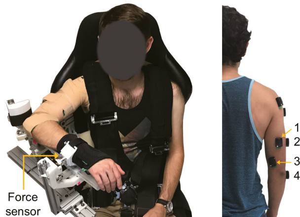
Figure 1. Experimental setup. (Left) Exoskeleton testbed. (Right) sEMG sensor placement: (1) long, (2) lateral, and (3) medial heads of the triceps brachii, and (4) anconeus muscles.
