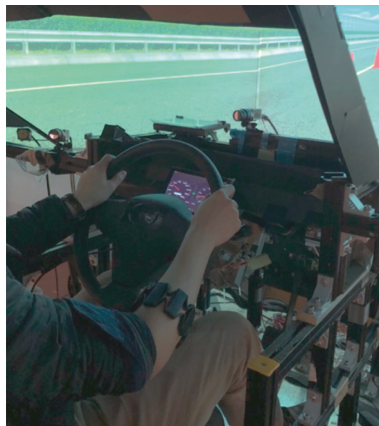
Figure 1. Active steering system and armband worn by driver to enable sEMG-based operation of a high-fidelity driving simulator.
