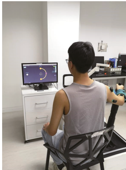
Figure 1. The upper limb movement experiment based on the rehabilitation robot.
