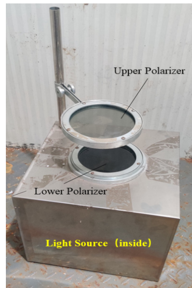
Figure 3. Ice crystal structure observation device.
