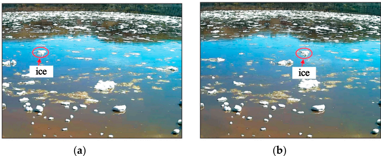
Figure 11. Manual extraction of ice position: (a) original position of target ice at 10:28 on 2 May 2016; (b) position of target ice after 10 s [13].
