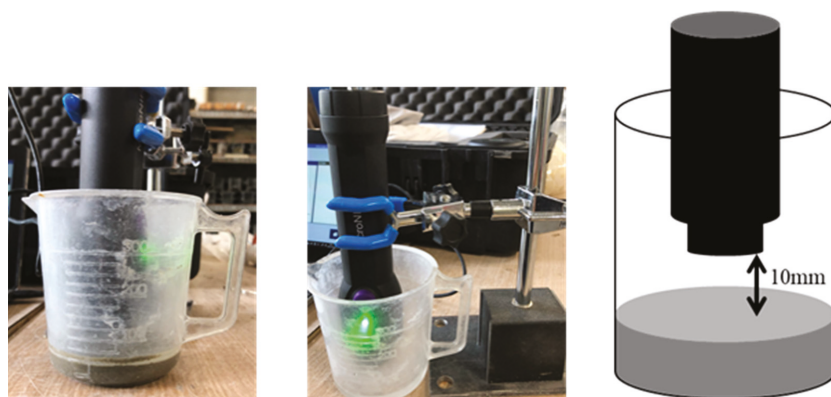
Figure 14. Spectral measurement immediately after mixing (cement paste).
