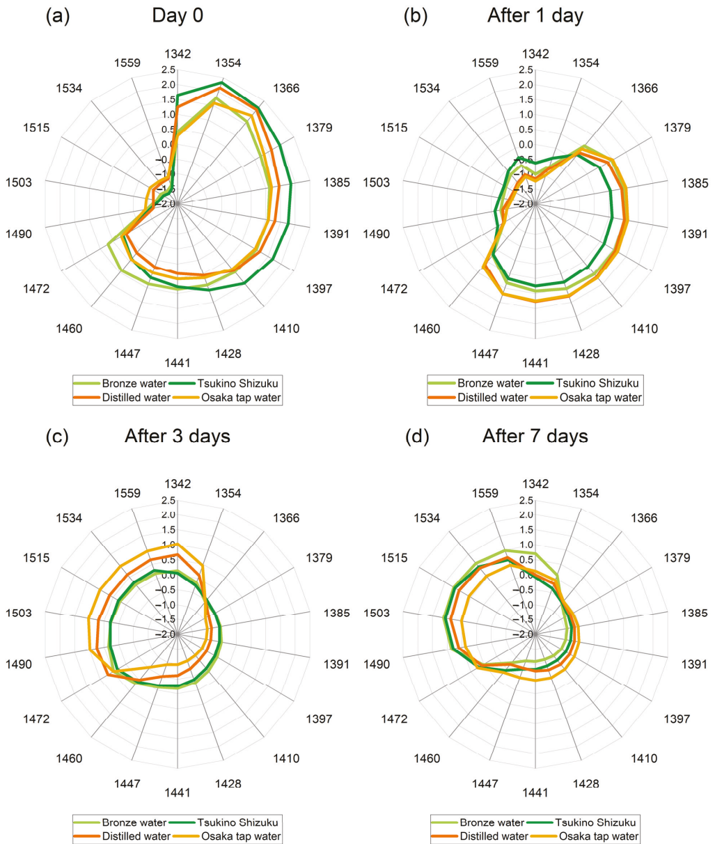
Figure 10. Aquagrams of cement paste and mortar grouped according to the time points when the measurements were performed: (a) Day 0—immediately after mixing of cement paste, (b) one day after the mortar was removed from the frame and left to cure, (c) three days after the mortar was removed from the frame and left to age, and (d) seven days after the mortar was removed from the frame and left to age. The aquagrams demonstrate the differences in water spectral patterns (WASPs) of cement mortar depending on the water used for mixing, and the aquagram profiles are colored accordingly.
