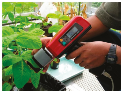
Figure 6. Acquiring soybean leaf spectra by handheld NIR spectrometer with a custom designed probe.
