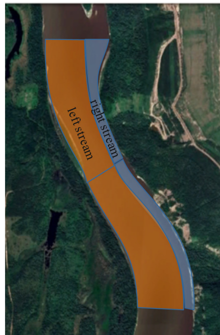
Figure 8. Discretising left and right stream along the Athabasca River modelling domain (map source: Google Earth).
