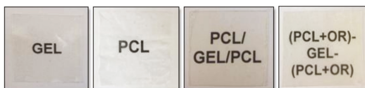
Figure 4. Contact transparency pictures, from left to right, GEL, PCL, PCL-GEL-PCL, and (PCL+OR)-GEL-(PCL+OR) films.
