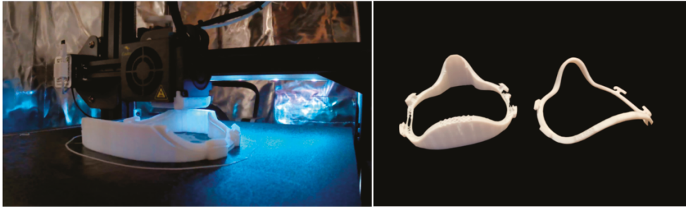
Figure 4. A 3D-printing process with a personal filament 3D-printer (left) and the Mask Fitter after printing and finishing.
