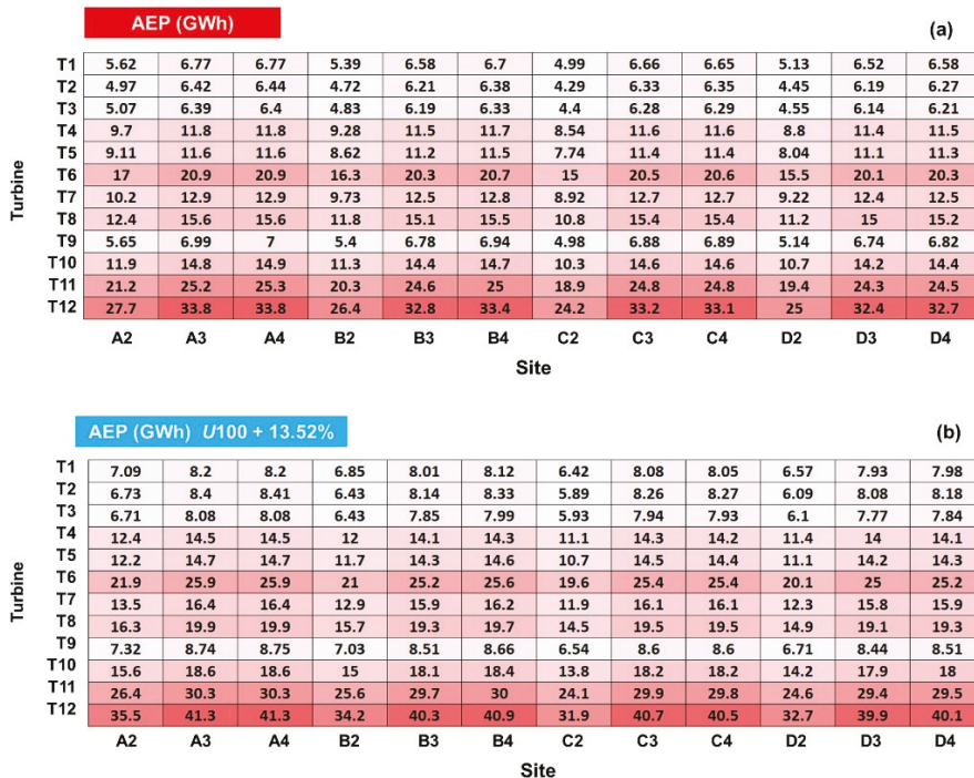
Figure 10. Annual Electricity Production (in GWh) expected to be provided by the wind turbines considered for the interval 2000–2019. Results indicated in terms of: (a) AEP—expected values based on ERA5 data; (b) adjusted AEP by considering an adjustment of the U_{100} time series (each value) by 13.52%.
