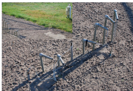
Figure 3. Measurement of soil moisture with the use of TDR/MUX/mpts and MIDL_GPRS data acquisition loggers at the Faculty Agro and Hydrometeorology Observatory.
