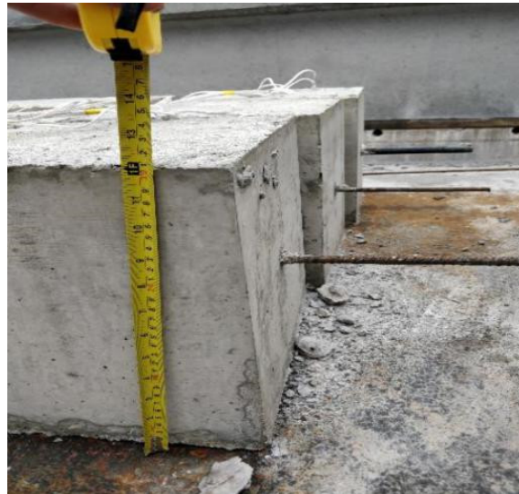
Figure 1. Reinforced concrete test specimens.
