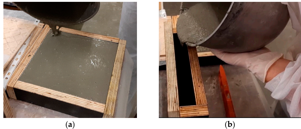
Figure 7. Casting of UHPFRC plates with moulds in (a) horizontal position; (b) vertical position.
