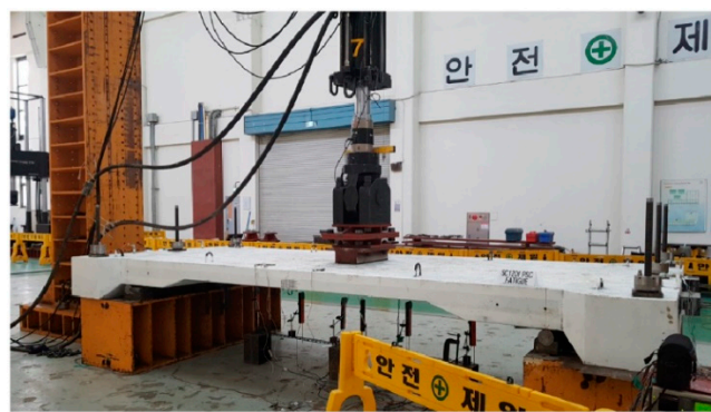
Figure 9. Fatigue testing of SC120f-PSC-JF specimen.
