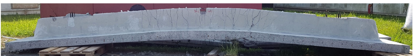
Figure 11. Example of deflected beam after testing.
