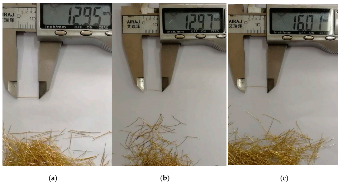
Figure 2. Steel fiber types: (a) 13SSF, (b) 13HSF and (c) 16HSF.
