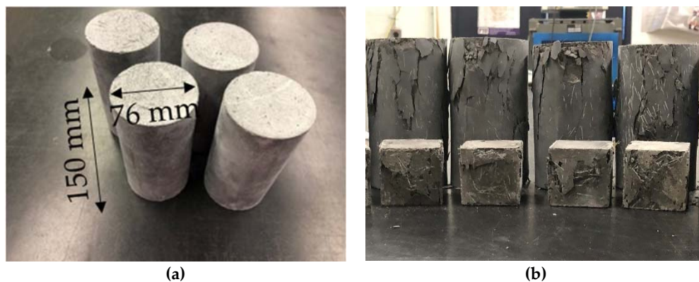
Figure 7. Compressive test specimens: (a) cylindrical specimens before the test; (b) cylindrical and cubical specimens after the test.
