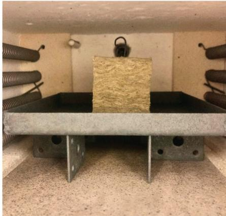
**Figure 3.** Test setup in the muffle oven.
