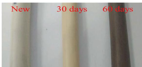
**Figure 1.** Digital photographs of polyvinyl chloride (PVC) sheaths before and after thermal aging.
