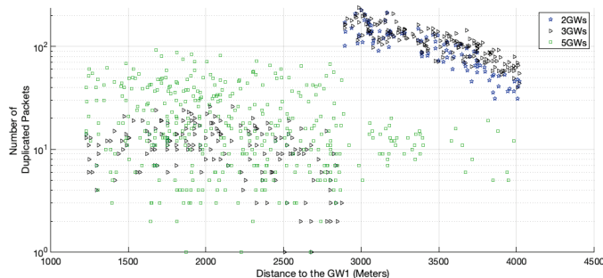
Figure 9. Number of duplicated packets per ED for a network with 2000 EDs using channel hopping protocol.
