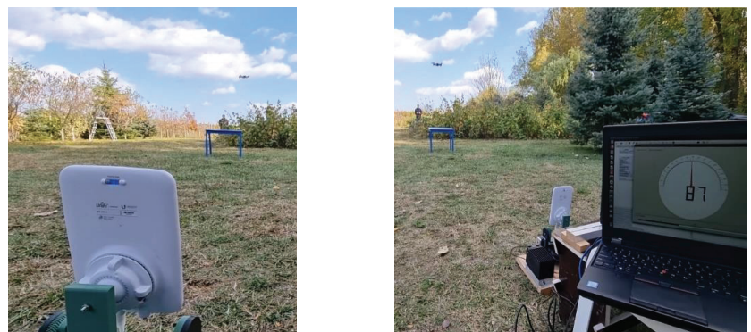
Figure 5. Tests performed using the DronEnd ground system (DJI Mavic AIR target drone). The estimated angle of incidence can be noticed.
