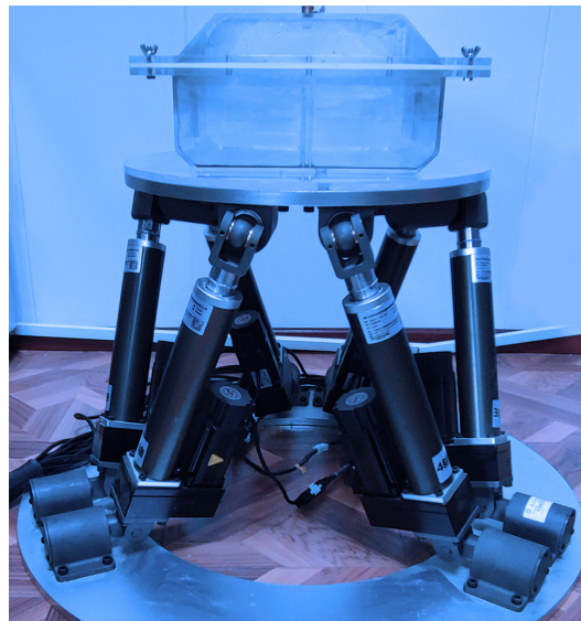
Figure 2. Six-degrees-of-freedom motion experimental platform.
