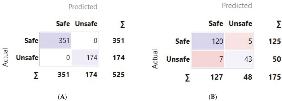
Figure 9. The AdaBoost model results for FOS classification: (A) Training and (B) Testing.
