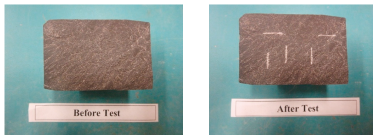
Figure 5. Example of rock surface conditions with rough surface (left over from BTS test) used for CAI test.
