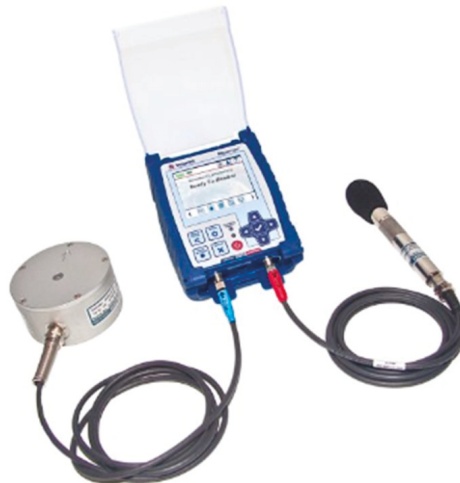
Figure 3. Instantel Micromate ISEE Std/XM seismograph.
