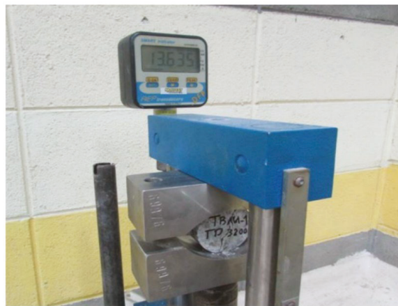
Figure 1. Failure of a sample under a BTS test [3].
