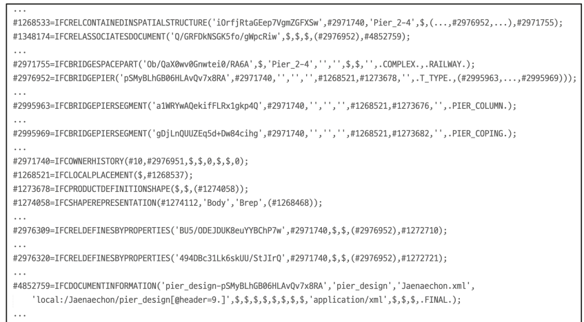
Figure 15. IPF (shown partially) generated using integrated assistant module related to Pier_2-4 object.
