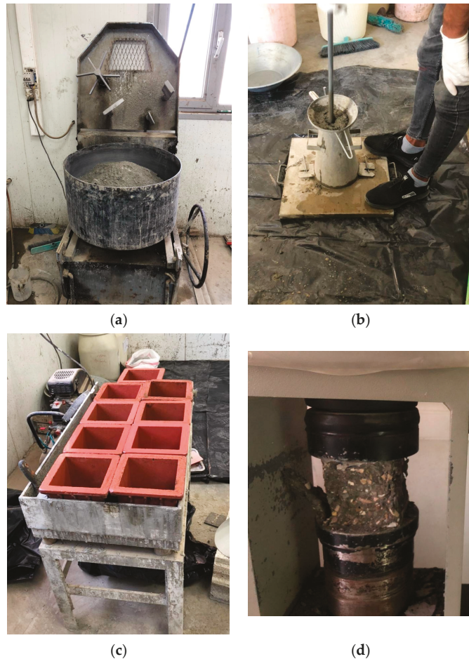
Figure 1. Experimental work (a) concrete mixer, (b) slump test, (c) cubic molds, (d) compressive strength test.
