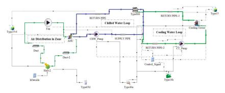
Figure 4. Water-cooled vapour compression cooling system simulated in TRNSYS.
