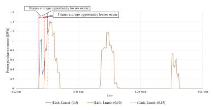
**Figure 15.** Changes in the power purchase amount when the initial inventory amount  $L_{init} = 0$  [kWh] and the maximum storage capacity  $L_{max} = 0$ , 5, 10 [kWh].
