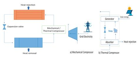
Figure 1. Schematic diagram of the conventional vapour compression cycle and the solar-driven vapour absorption cycle.
