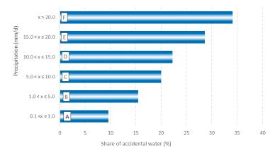
**Figure 5.** Percentage share of accidental water in the total amount of wastewater flowing into the wastewater treatment plant in Nowy Targ against the background of characteristic precipitation events.
