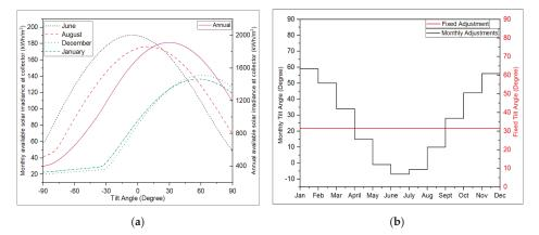
Figure 13. (a) Variation of solar irradiance as a function of collector tilt angle; (b) monthly optimized collector tilt angles.
