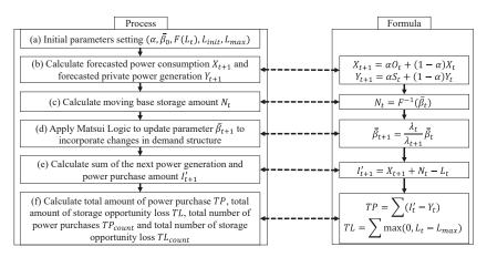
Figure 4. Procedure for applying the on-demand DSMM to renewable power generation.
