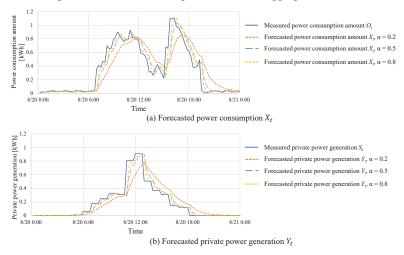
**Figure 8.** Predicted vs. measured power consumption amount  $X_{t+1}$  power generation  $Y_{t+1}$  based on  $\alpha$  values of 0.2, 0.5, and 0.8.
