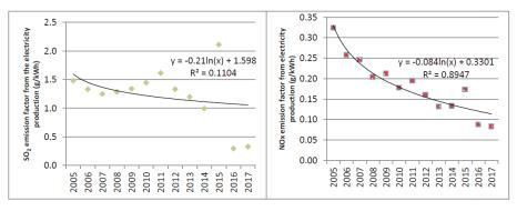
Figure 3. The development of the course of SO<sub>2</sub> (left) and NO<sub>x</sub> (right) emission factor in the production of electricity in the period 2005–2017 in the Slovak Republic.
