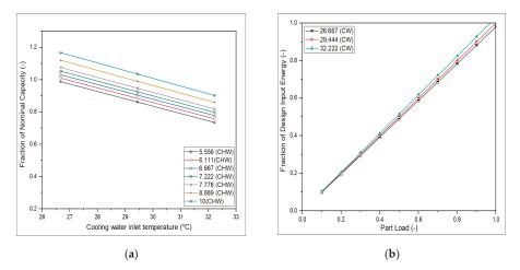
**Figure 6.** (a) Fraction of nominal capacity with varying cooling water inlet temperature at different chilled water temperatures for absorption cooling system (ACS); (b) fraction of design input energy at different part load ratio for ACS.
