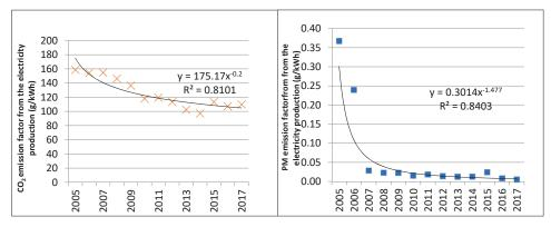
Figure 2. The chain of  $CO_2$  (left) and PM (right) emissions production in transport with the use of fossil fuels (direct and indirect emissions).
