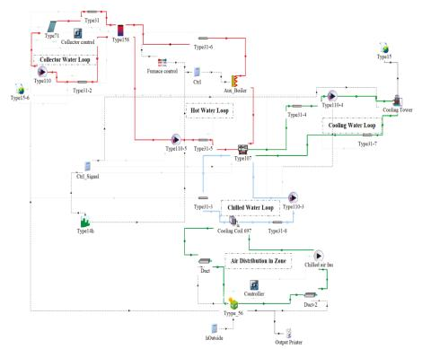
Figure 3. Solar absorption cooling system simulated in TRNSYS.
