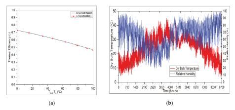
**Figure 7.** (a) Comparison of collector efficiency curve (simulation vs. experimental data reported by the collector's manufacturer at  $G = 1000 \text{ W/m}^2$ ); (b) daily temperature and humidity variation for Lahore, Pakistan.
