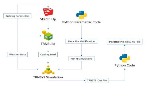
Figure 2. Simulation and parametric study methodology.
