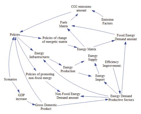
Figure 1. Flow diagram of the energy system and production of carbon emissions in Ecuador (adapted from [18]).
