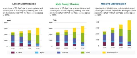
Figure 5. Electricity supply by technology in the different scenarios (TWh).
