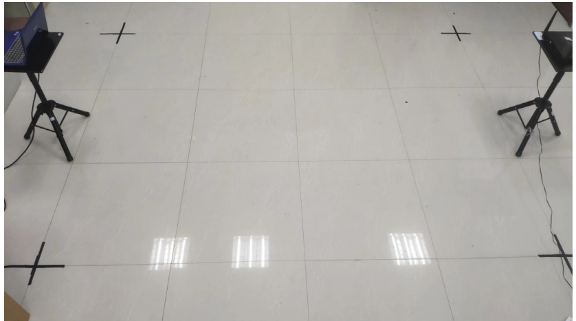
Figure 2. The area where the CSI data were collected. The crossbelt marks the boundary of the area, which is 2.4 m \times 3.2 m in size.
