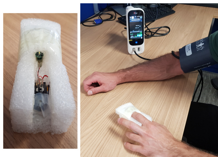
Figure 5. An example of BP and PPG setup for data acquisition on volunteers at STMicroelectronics.
