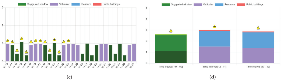
Figure 6. The UFM scheduler result, providing the operator with potential timeframes (green color) during which to schedule a specific maintenance operation. The final activity index is decomposed in all its constituent values, contributing to the final index. The analysis considers a period of one month, starting from 10 November 2021. (a) Equal cost timeframes proposed by the scheduler for a maintenance operation in Via Indipendenza X, Bologna, Italy. (b) Identified non-binding interference for a maintenance operation in Via Zamboni, Bologna, Italy, in the interval [10, 23]. (c) Equal cost timeframes, vehicular data only, proposed by the scheduler for a maintenance operation in Via Zamboni. (d) Scheduling of an urgent intervention in Via Zamboni, relying on the next-day prediction of the activity index.
