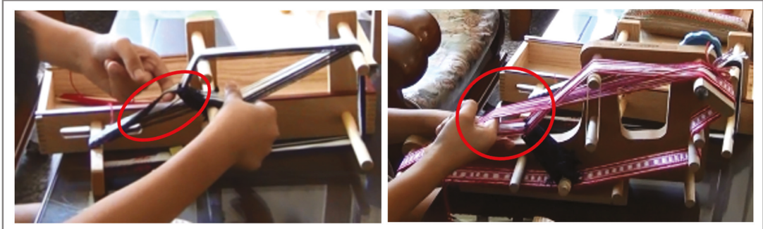
Figure 9. “Shed” on both mini-looms. ((Left): smaller on a modern weaving box; (Right): larger on a New Zealand ribbon loom).
