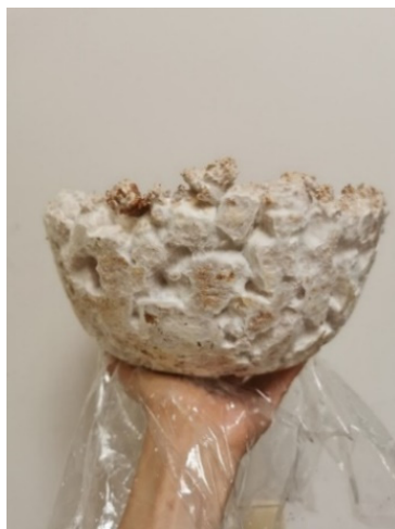
Figure 9. Mycelium-based composite: rough texture, deriving from substrate fragmentation (design and photo: A. Bonenberg).
