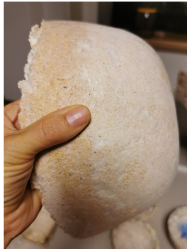
Figure 8. Mycelium-based composite: smooth texture, with visible fibres (design and photo: A. Bonenberg).
