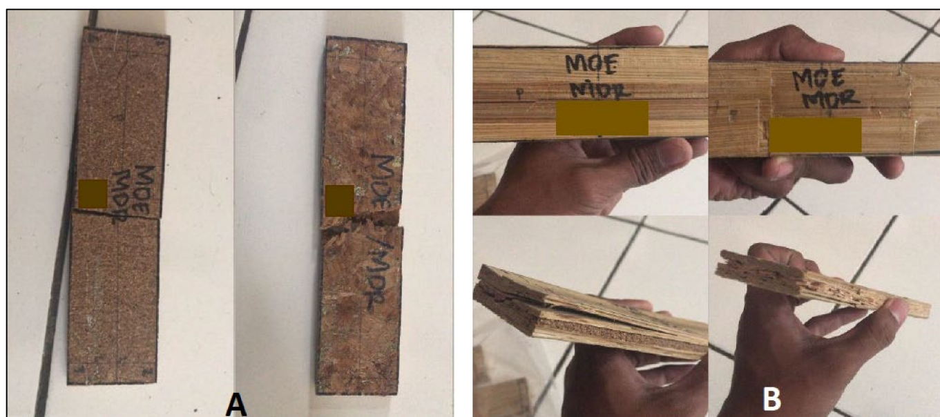
Figure 15. The appearance of damage in samples in MOE and MOR testing: nonstrand-coated board (A), and strand-coated board (B).
