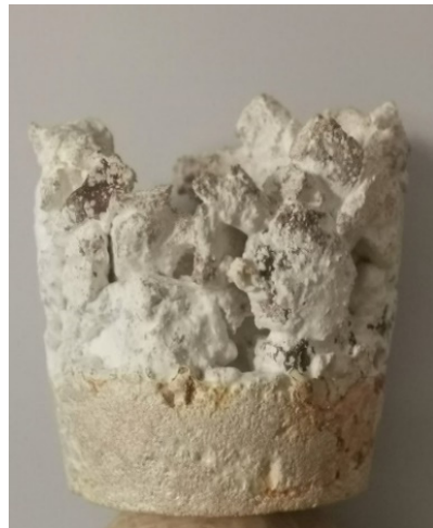
Figure 10. Mycelium-based composite: smooth and rough textures, combined in one object (design and photo: A. Bonenberg).
