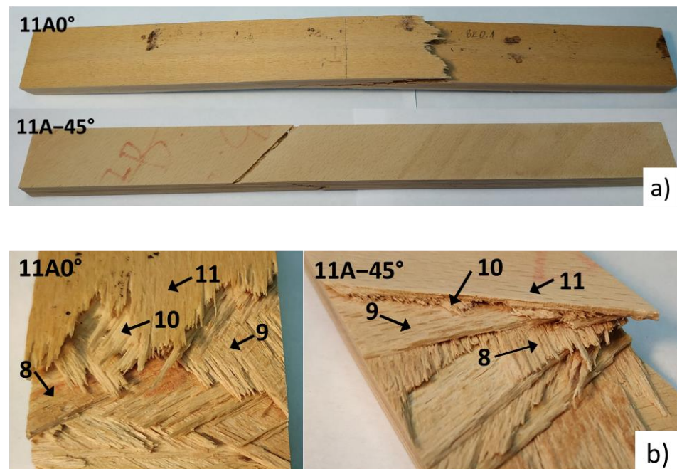
Figure 7. 4-point bending specimens 11A0° and 11A-45°: (a) Whole specimens; (b) detail of the specimen underside with layer numbering.
