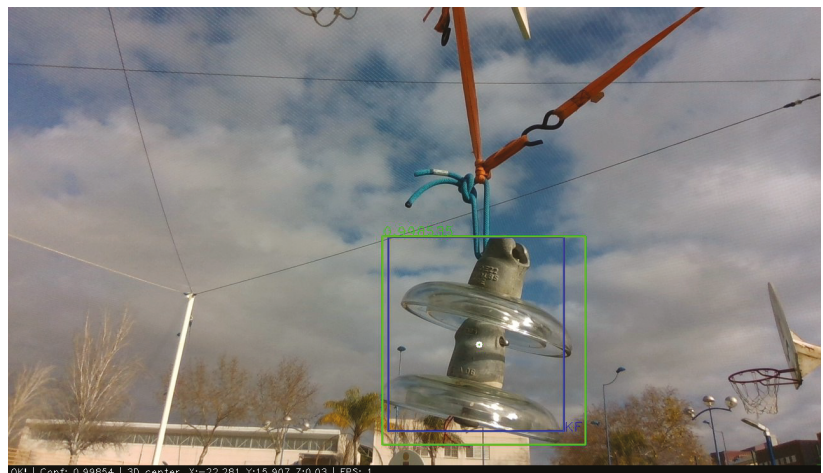
Figure 7. Insulator detection using YOLO v4 Tiny with TensorRT implementation (green bounding box) and tracker result (blue bounding box).
