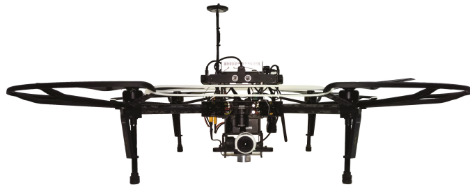
Figure 5. The robot developed for our project. The figure shows our DJI Matrice 100 quadrotor equipped with the indoor testing parts (DJI Guidance System and the propeller guards), as well as the DJI Zenmuse X3 Gimbal and Camera system, the SF30 altimeter, and the DJI Manifold onboard computer.
