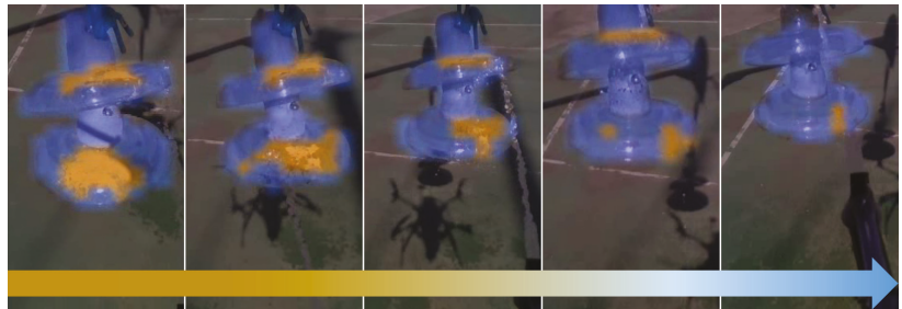
Figure 14. Evolution of soiled areas in the insulator.
