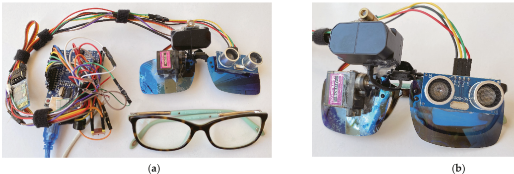
Figure 7. (a) LidSonic V2.0 device and a glass (b) LidSonic V2.0 device mounted into a glass frame.
