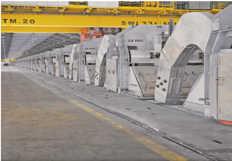
Figure 1. System’s working environment characterised by a high magnetic field up to 300–500 Gauss, ambient temperature up to 60 °C, high pot shell temperature varying between 120 °C and 500 °C, high relative humidity up to 100%, and concrete debris on the floor.
