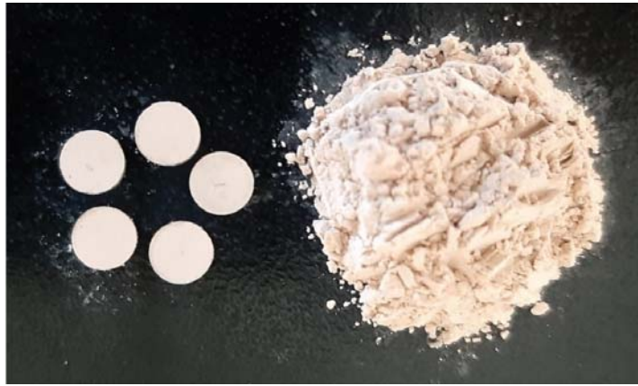
Figure 1. Rhyolite compressed disks at 3 tons.
