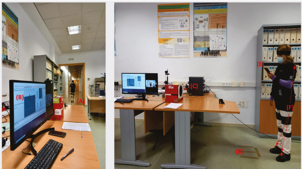
Figure 2. Instrumentation and experiment environment. (A) 24-m-long corridor the participants must walk. (B) Monitor where the movement of the person is visualized in real time. (C) Computer with motion capture software. (D) Start position marks. (E) Personal mobile device. (F) Some of the MTw IMUs.
