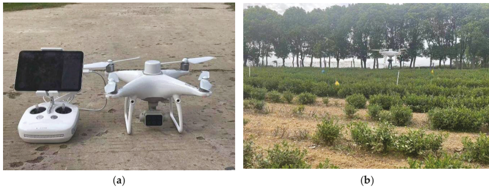
Figure 2. Types of UAVs and sensors used in this study: (a) quad-rotor UAV with RGB sensor, DJI Phantom 4 RTK, (b) flying operations.
